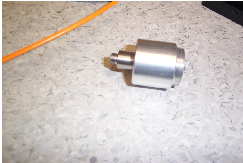
Figure 4.4: Cylindrical tube with collimator at left-most end and filter inside
