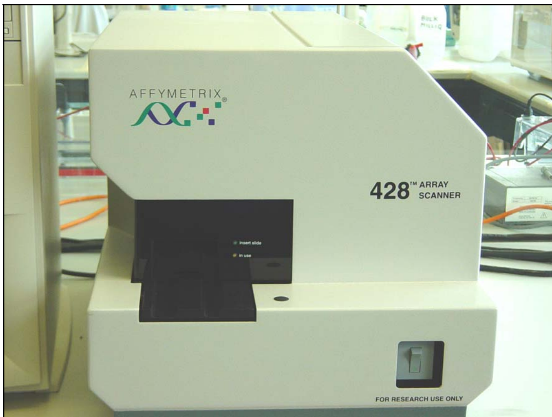
Figure 3.9 The Affymetrix® 428™ (Santa Clara, CA ) array scanner at RMIT University used for microarray scanning.
