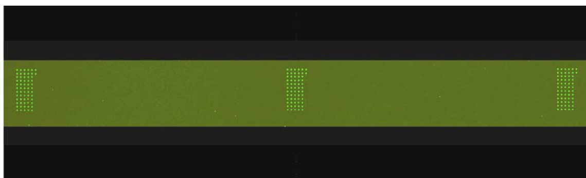
Figure 3.8 A non-hybridised microarray slide showing the three sub-grids printed per slide.
