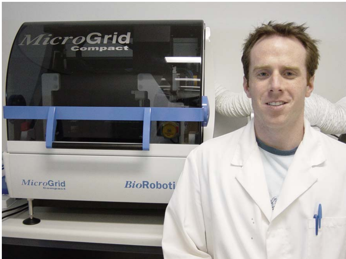
Figure 1.7 A BioRobotics® MicroGrid II Compact array printing robot (Genomic Solutions, Ann Arbor, MI).
