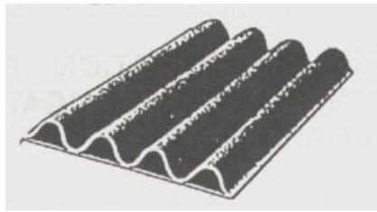
Figure [1.1.2] – Single facer board reproduced from Wright et al. [1]
