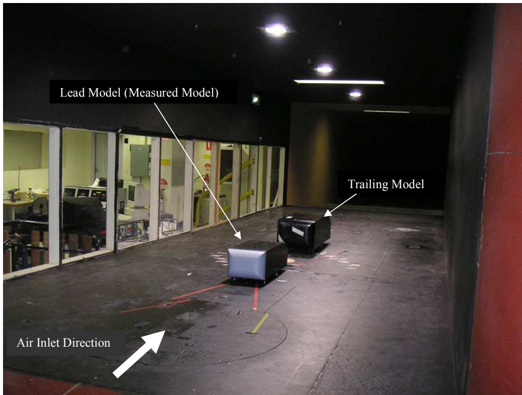
Figure 42. Experimental setup for two scales of Ahmed models at RMIT Industrial Wind Tunnel (IWT)
