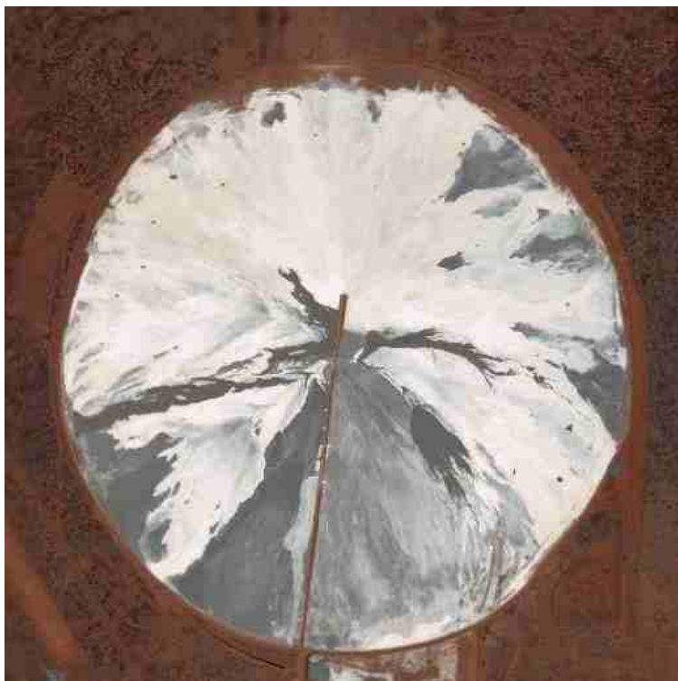
Figure 137. An aerial photograph of the Sunrise Dam stack. The dark areas on the stack surface show the locations of recently deposited tailings. (Picture provided by Google Earth ©)
