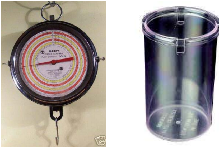
Figure 22. Marcy density scale (left) and 1 litre plastic bucket with notch weirs (right)
