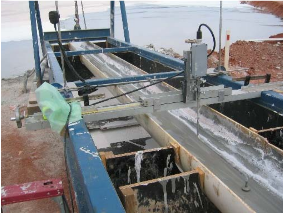
Figure 17. Traversing jig with the velocity probe attached. Note that slurry flow is very low.
