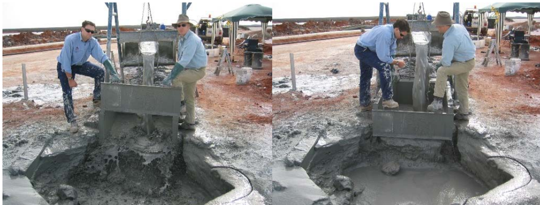
Figure 14. Flow measuring box with gate open (left) and closed (right)
