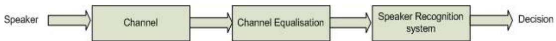
Figure 1.1: Channel equalisation directly after channel (before data is entered into speaker recognition system)
