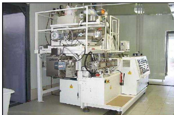
Figure 2.1: The food cooking extruder machine
