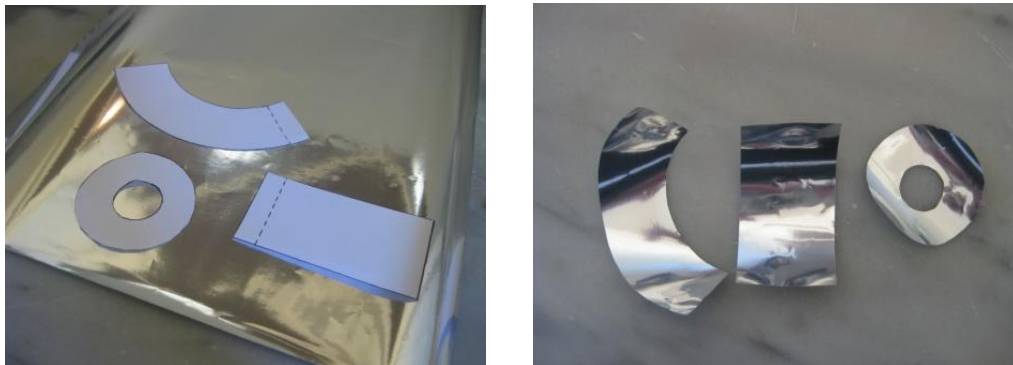
Fig. 36: Cutting pattern pieces for prime focus antenna feed horn components
