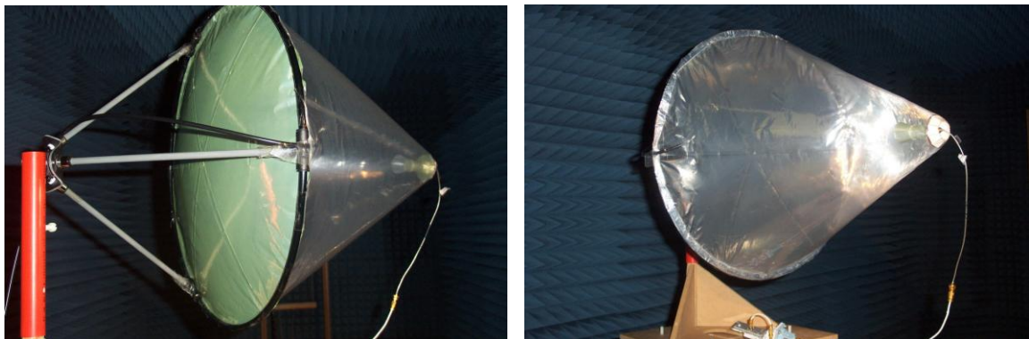
Fig. 56: Inflatable antenna with gossamer horn mounted on rigid frame in anechoic chamber
