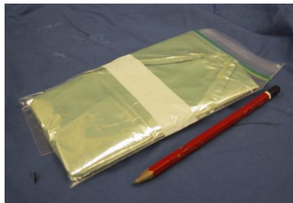
Fig. 57: Inflatable antenna with gossamer horn stowed for travel
