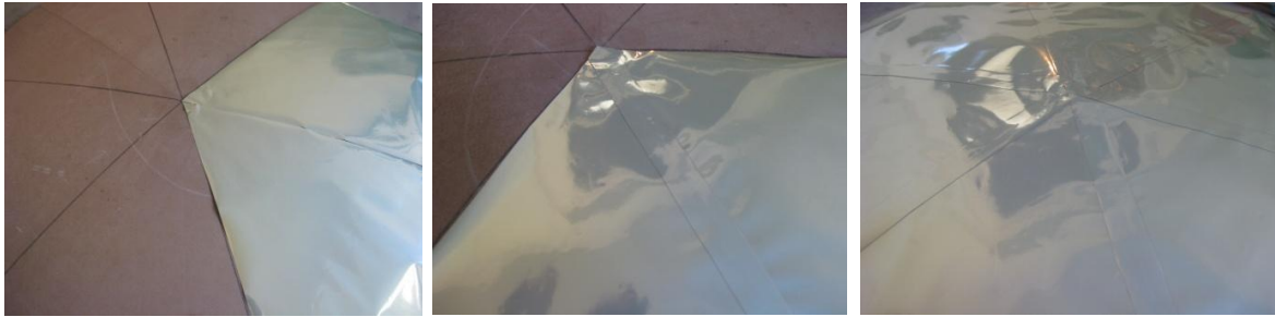
Fig. 108: Assembly of parabolic reflector from thin film gores using a plug.
