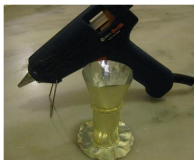
Fig. 41: Hot glue gun used to assemble feed horn pieces
