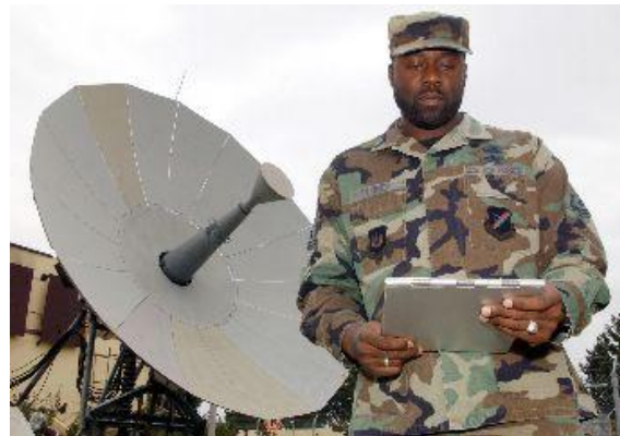
Fig. 4: Typical petal deployable parabolic dish antennas (image courtesy Thales and US of DoD)
