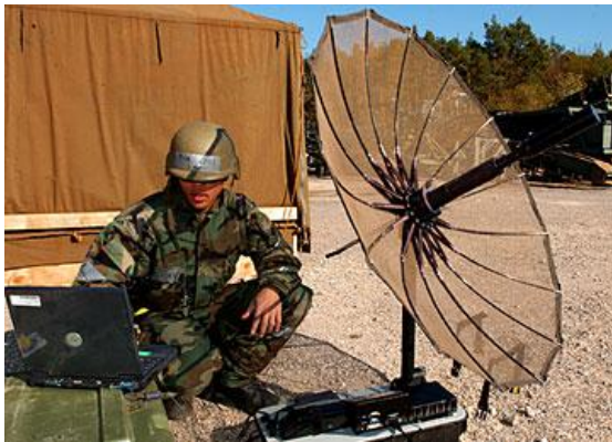
Fig. 3: Typical articulated mesh, or umbrella, parabolic dish antenna (image courtesy of US DoD)
