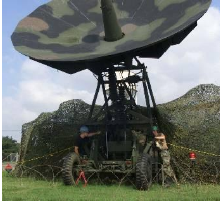
Fig. 1: Typical military Communications-on-the-Halt (COH) ground station (image courtesy of US DoD)
