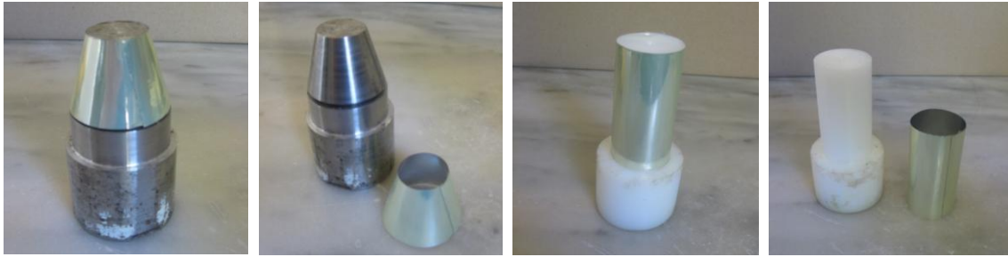
Fig. 37: Assembly of individual horn components with the assistance of shaped plugs
