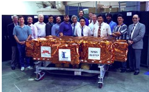
Fig. 12: L'Garde Inflatable Antenna Experiment (IAE) stowed ready for launch (image courtesy of L'Garde)
