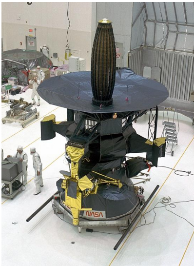
Fig. 6: Galileo High Gain Antenna in the stowed position (image courtesy of NASA)
