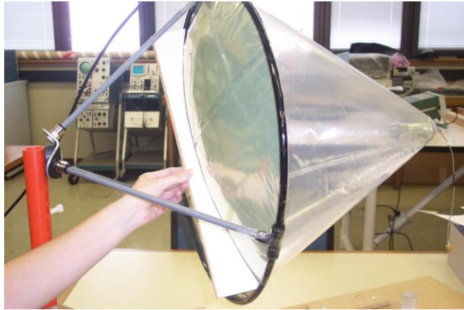
Fig. 54: Inflatable antenna with gossamer horn mounted on rigid frame
