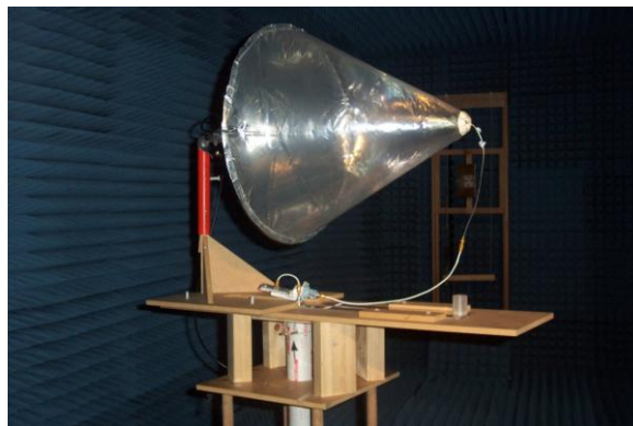
Fig. 55: Inflatable antenna with gossamer horn mounted on rigid frame in anechoic chamber
