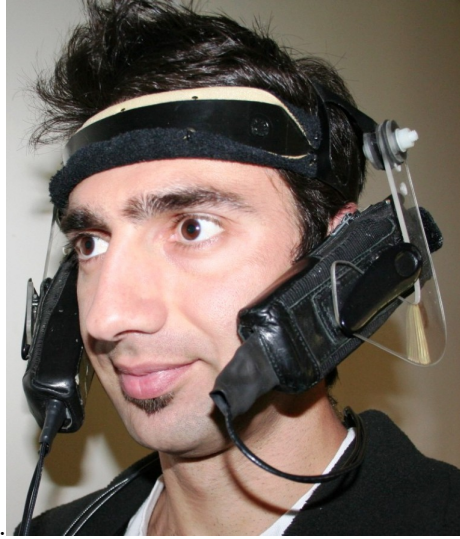
Figure 5.4.: A depiction of the mobile phone head cradle which can support two mobile phone devices in the standard ear to mouth position. Here only one device is shown.
