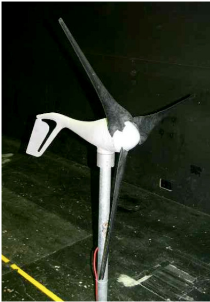
Figure C1: AIR 403 aerogenerator install inside RMIT Industrial Wind Tunnel.
