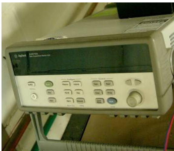
Figure 51: Agilent 34970A data acquisition unit, which takes data from all transducers and sends this information to the PC. It also take commands from the PC to control the contactor unit.
