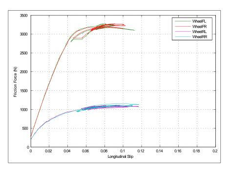
Figure 6.15: Plot of longitudinal slip vs. tyre friction force on high friction surface  $(\mu = 0.5)$
