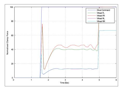
Figure 4.22: Case A : Applied clamp forces by the controller during an emergency braking manoevure (1.5 sec -5 sec). A spike braking input is applied by the driver model (driver cmd) at 1.5 sec: (p = 0.45)
