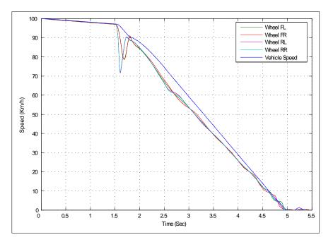
Figure 4.20: Case A : plot of vehicle and wheel speeds during an emergency braking manoeuvre: a spike braking is applied at 1.5 sec, and a parameter p is tuned at 0.45
