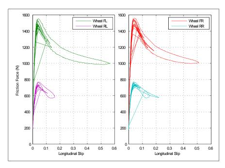
Figure 6.33: Characteristic friction force curve of front and rear wheels for ABS braking stop on a low friction surface ( $\mu = 0.2$ )
