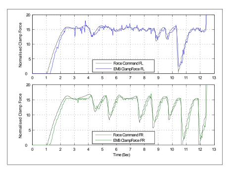
Figure 6.19: Amplified view of front EMB caliper response to the force command input
