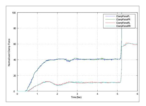
Figure 6.9: Measured clamp forces by the EMB calipers for a high friction surface  $(\mu = 0.85)$  with the parameter p tuned at 0.35 : Initial braking is applied around 0.5 sec
