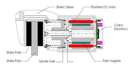
Figure 1.3: Cross-sectional view of EMB
