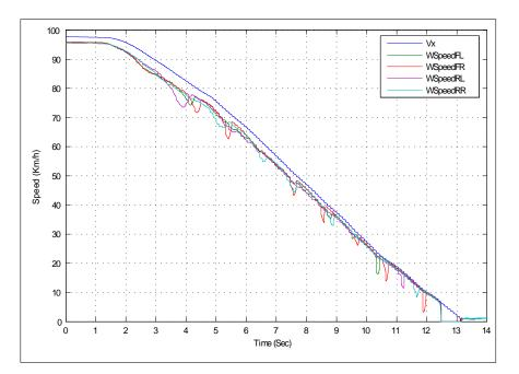
Figure 6.16: Plot of simulated vehicle speed (Vx) and wheel speeds (WSpeed) on a low friction surface ( $\mu = 0.2$ ): Initial vehicle speed of 100 km
