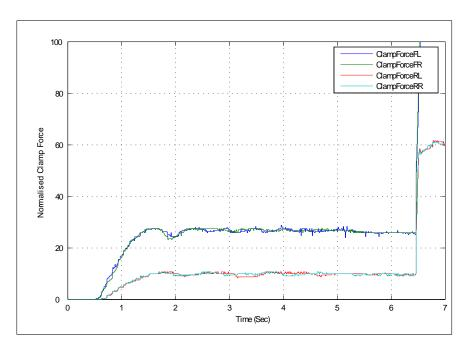
Figure 6.13: Measured clamp force by the EMB caliper for a high friction surface  $(\mu=0.5)$
