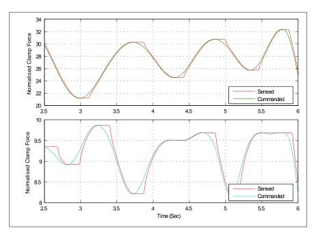
Figure 4.28: Amplified view of responses by the EMB caliper model (Sensed) to the commanded clamp force (Commanded) from the wheel slip controller : (a) front left brake caliper; (b) rear left brake caliper :Medium friction surface ( $\mu = 0.5$ ); (p = 0.25)
