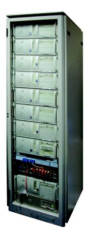
Figure 4.1: Picture of Real-time Simulation Cluster: comprises of 7 real-time simulation units constructed based on PC, reflective memory network, including reflective memory network switch and host PC
