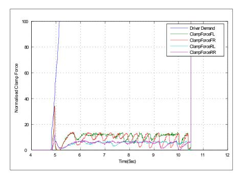
Figure 6.32: Plot of measured clamp forces by EMB brake calipers (ClampForce FL,FR,RL,RR) and driver brake request (Force Demand) during ABS braking for a low friction surface ( $\mu = 0.2$ )
