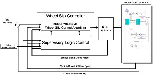
Figure 3.2: Local wheel slip controller configuration
