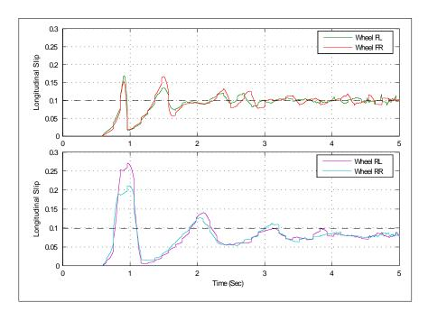
Figure 6.23: Simulated longitudinal slip responses of front and rear wheels w.r.t optimal slip setpoint of 0.1 (dashed line) on a high friction surface ( $\mu = 0.85$ ) for ABS braking manoeuver:
