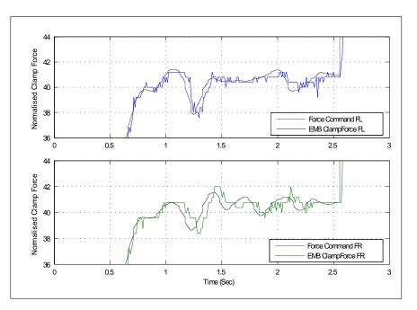
Figure 6.10: Amplified view of measured clamp forces by the front EMB calipers for a high friction surface ( $\mu = 0.85$ ) with the parameter p tuned at 0.35
