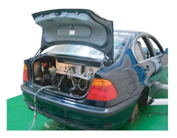
Figure 6.2: Rear view of prototype brake-by-wire vehicle in HiL simulation set-up
