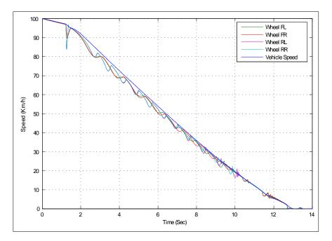
Figure 4.30: Plot of vehicle and wheel speeds during an ABS braking manoeuvre on a low friction surface ( $\mu = 0.2$ ): a step braking is applied at 1.5 sec ; (p = 0.2)
