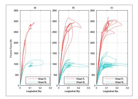
Figure 4.14: Plot of type friction forces vs longitudinal slips on high friction surface  $(\mu = 0.85)$ : (a) p = 0.2 (b) p = 0.4 (c) p = 0.8
