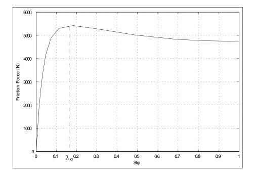
Figure 1.1: Type friction curve
