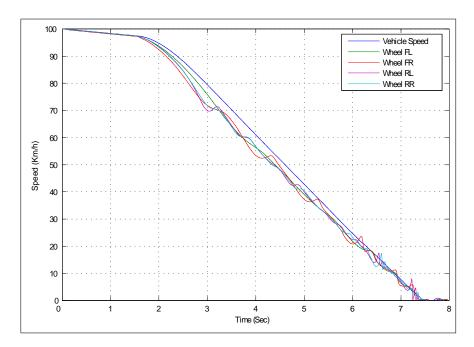
Figure 4.16: Plot of vehicle and wheel speeds on a medium friction surface ( $\mu = 0.5$ ) with with p value of 0.2
