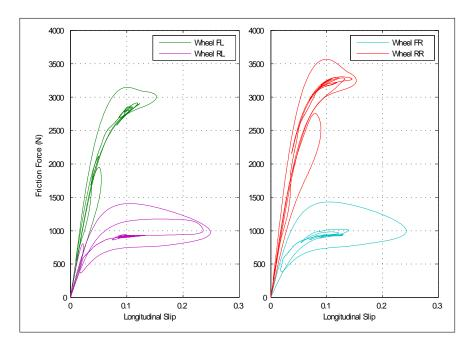
Figure 4.24: Characteristic friction curve for a high friction surface ( $\mu = 0.85$ ) during an ABS braking manoeuvre
