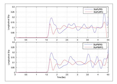
Figure 5.4: Comparison of front wheel slip response w.r.t optimal slip level (dashed line) of 0.1 on a high friction surface ( $\mu = 0.85$ )
