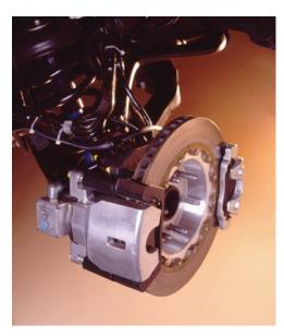
Figure 1.4: Photo of EMB fitted in the vehicle.
