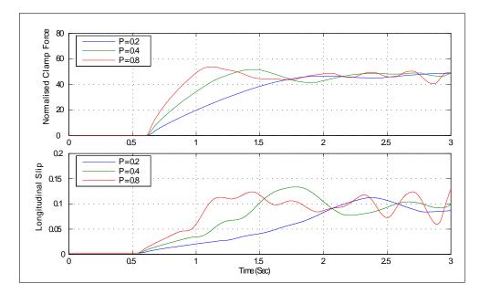
Figure 4.10: Commanded clamp forces (top) and longitudinal slip response of a front left wheel (bottom) on a high friction surface ( $\mu = 0.85$ ) with varying value of parameter p
