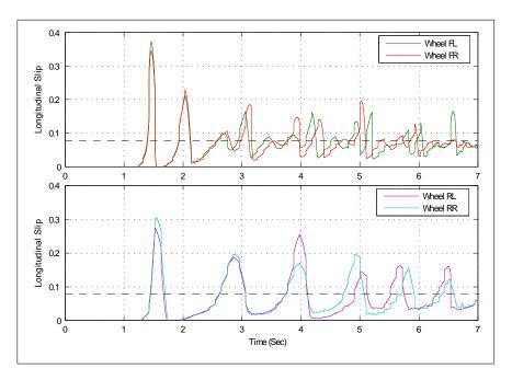
Figure 6.27: Simulated longitudinal slip responses of front and rear wheels w.r.t optimal slip setpoint of 0.08 (dashed line) on a medium friction surface ( $\mu = 0.5$ ) for ABS braking manoeuver:
