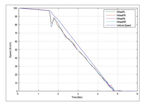
Figure 5.3: Plot of vehicle and wheels speed on a high friction surface ( $\mu = 0.85$ ). Spike braking is applied at 1.5 sec: Model Predictive Control
