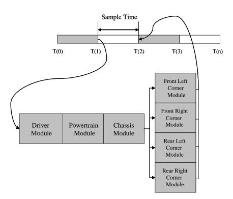
Figure 4.6: A revised execution list of the distributed vehicle model.
