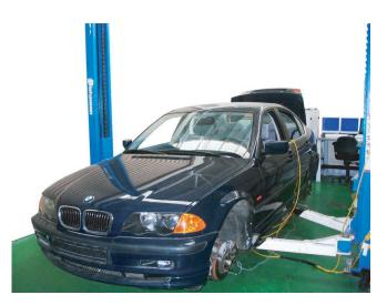
Figure 6.1: Front view of prototype brake-by-wire vehicle in HiL simulation set-up
