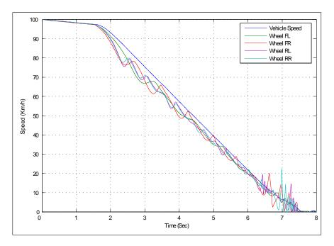
Figure 4.17: Plot of vehicle and wheel speeds on a medium friction surface ( $\mu = 0.5$ ) with p value of 0.4
