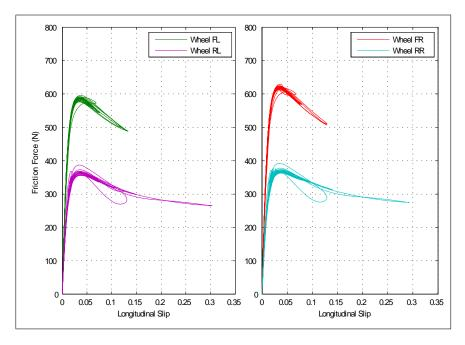
Figure 4.34: Characteristic friction curve for a low friction surface ( $\mu = 0.2$ ) during an ABS braking manoevure
