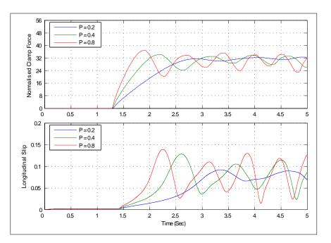
Figure 4.15: Plot of commanded clamp forces (top) and longitudinal slip response of a front left wheel (bottom) on a medium friction surface ( $\mu = 0.5$ ) with varying value of parameter p
