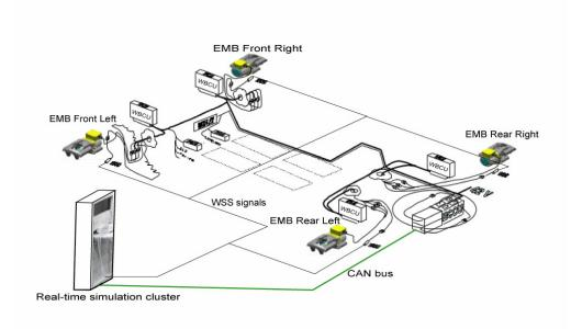
Figure 6.4: An overview of hardware-in-the-loop simulation set-up
