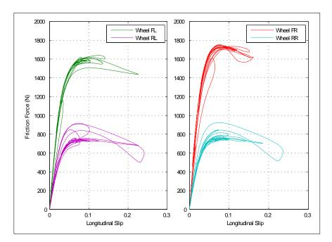
Figure 4.29: Characteristic friction curve for a medium friction surface ( $\mu = 0.5$ ) during an ABS braking manoevure
