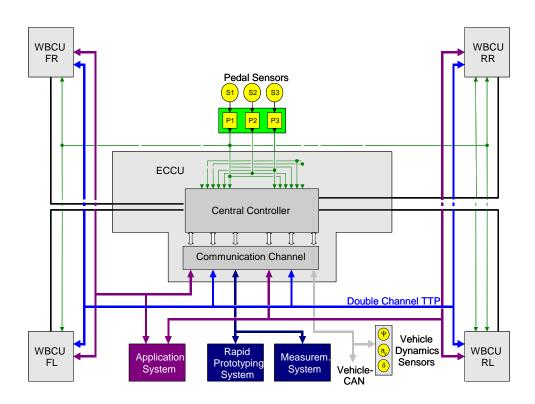
Figure 3.1: Control system architecture of BBW system
