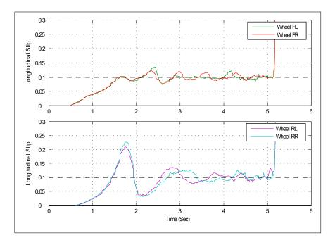
Figure 6.8: Simulated longitudinal slip responses of front wheels (FL,RL) and rear wheels (RL,RR) w.r.t slip setpoint of 0.1 (dashed line) on a high friction surface ( $\mu = 0.85$ ).
