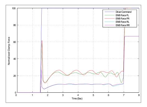
Figure 4.27: Plot of clamp force inputs by the slip controller during an ABS braking manoevure and the spike braking input from the driver model (driver cmd) at 1.5 sec: Medium friction surface ( $\mu = 0.5$ ); (p = 0.25)
