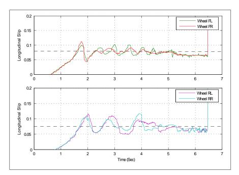
Figure 6.12: Simulated longitudinal slip responses of front wheels (FL,RL) and rear wheels (RL,RR) on a high friction surface ( $\mu = 0.5$ ) w.r.t slip set point of 0.08 (dashed line)
