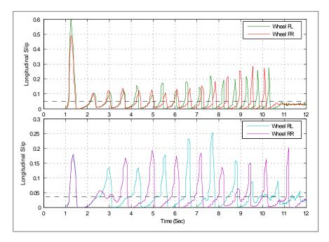
Figure 6.31: Simulated longitudinal slip responses of front and rear wheels w.r.t optimal slip setpoint of 0.05 (dashed line) on a low friction surface ( $\mu = 0.2$ ) for ABS braking manoeuver:
