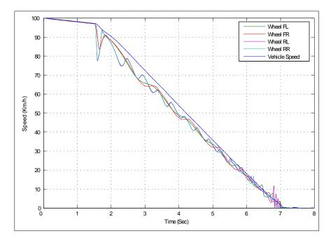
Figure 5.9: Plot of vehicle and wheels speed on medium friction surface ( $\mu = 0.5$ ) : MPC control
