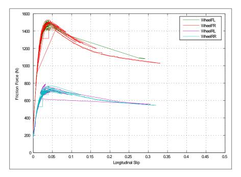
Figure 6.21: Plot of longitudinal slip vs. tyre friction force on low friction surface  $(\mu = 0.2)$
