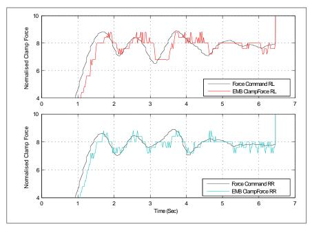
Amplified view of measured clamp force responses from the rear EMB calipers to the force command input
