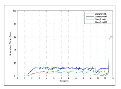
Figure 6.18: Measured clamp force by the EMB caliper for a low friction surface  $(\mu=0.2)$
