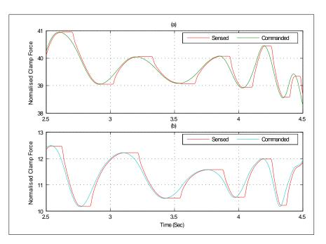
Figure 4.23: Case A: Amplified view of EMB simulation model responses (Sensed) to wheel slip controller force command inputs (Commanded) : (a) front left brake caliper; (b) rear left brake caliper : High friction surface ( $\mu = 0.85$ )
