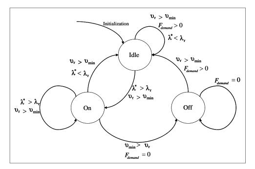
Figure 3.3: Wheel slip control state machine: Instantaneous slip  $(\lambda^*)$ , Slip threshold  $(\lambda_r)$ , Vehicle speed  $(v_r)$ , Minimum vehicle speed  $(v_{\min})$ , Driver force demand  $(F_{demand})$ .
