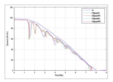
Figure 6.26: Plot of simulated vehicle (Vx) and wheel speeds (WSpeed) on a medium friction surface ( $\mu = 0.5$ ) for ABS braking manouevure.
