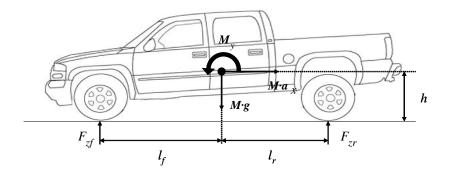
Figure 2.1: Loads acting on the longitudinal vehicle model during braking.
