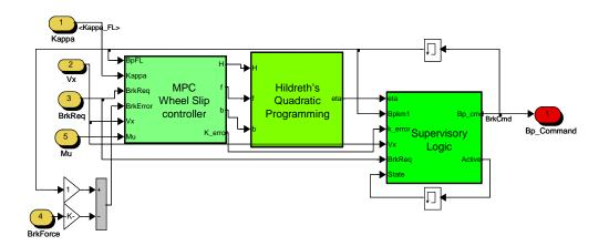
Figure 4.9: Simulink representation of the local wheel slip controller
