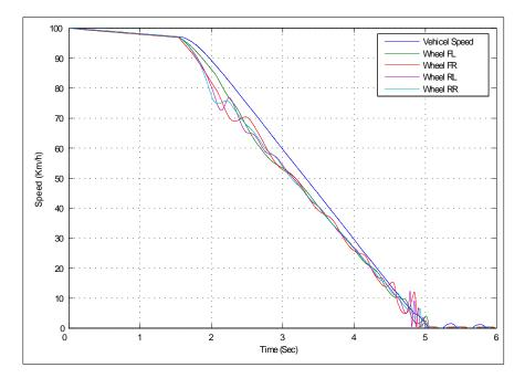
Figure 4.12: Plot of vehicle speed and wheel speeds on a high friction surface ( $\mu = 0.85$ ) with with p value of 0.4
