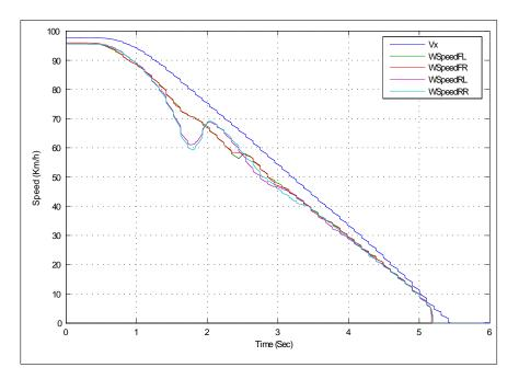
Figure 6.7: Plot of simulated vehicle speed (Vx) and wheel speeds (WSpeed) on a high friction surface ( $\mu = 0.85$ ) with the parameter p tuned at 0.35
