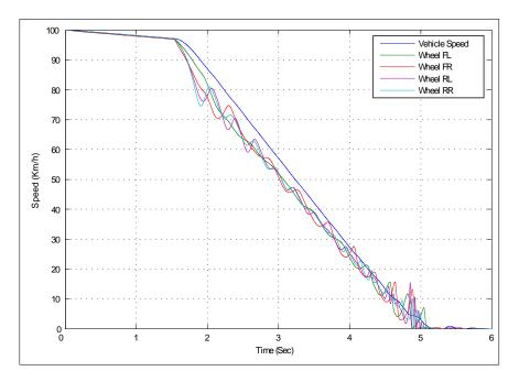
Figure 4.13: Plot of vehicle speed and wheel speeds on a high friction surface ( $\mu = 0.85$ ) with p value of 0.8
