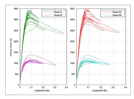
Figure 6.29: Characteristic friction force curve of front and rear wheels for ABS braking stop on medium friction surface ( $\mu = 0.5$ )
