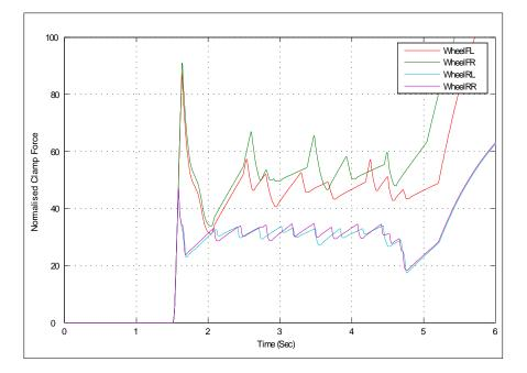
Figure 5.6: Response of EMB caliper model to force command signal generated by the PID controller, ( $\mu = 0.85$ ): When the slip value exceeds the threshold (see Figure 5.4 and 5.5) after 1.5 sec, the controller is turned on to reduce the clamp force to stabilise the slip value. Period between 2 and 5 sec, the brake clamp force are modulated by the PID controller to stabilise the slip at the optimal point. After 5 seconds, when the vehicle came to a full stop, the controller is turned off.
