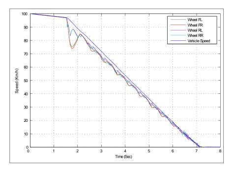
Figure 5.8: Plot of vehicle and wheels speed on medium friction surface ( $\mu = 0.5$ ) : PID control
