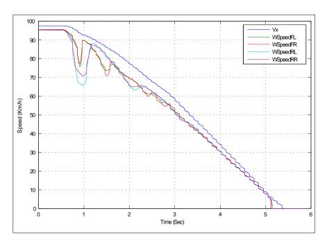
Figure 6.22: Plot of simulated vehicle (Vx) and wheel speeds (WSpeed) on a high friction surface ( $\mu = 0.85$ ) for ABS braking manouevure.
