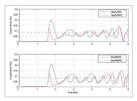
Figure 5.10: Comparison of front wheel slip response w.r.t optimal slip level (dashed line) of 0.08 on high friction surface ( $\mu = 0.5$ )
