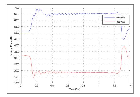
Figure 2.2: Variation of normal force  $(F_z)$  on front and rear wheels during step braking
