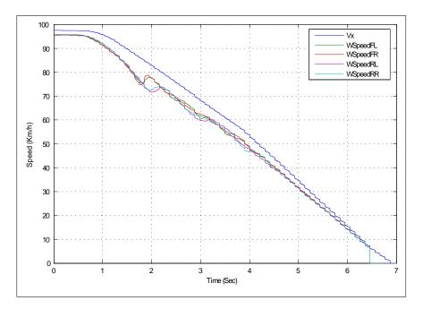
Figure 6.11: Plot of simulated vehicle speed (Vx) and wheel speeds (WSpeed) on a high friction surface ( $\mu = 0.5$ ): Initial vehicle speed of 100 km/h
