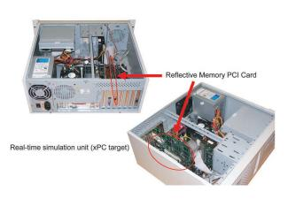
Figure 4.2: Fitted view of reflective memory card in real-time simulation unit
