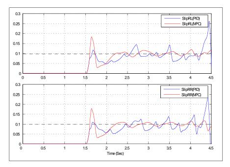
Figure 5.5: Comparison of rear wheel slip response w.r.t optimal slip level (dashed line) of 0.1 on a high friction surface ( $\mu = 0.85$ )
