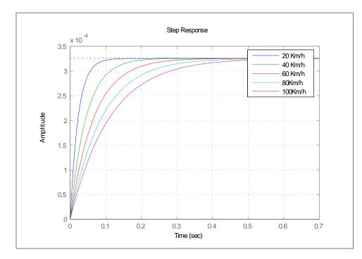
Figure 2.5: Step response of slip dynamic for speed from 20 Km/h to 100Km/h
