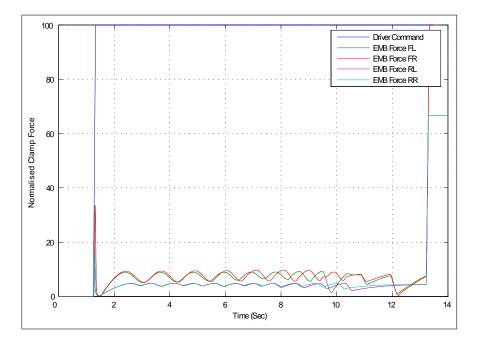
Figure 4.32: Plot of clamp force inputs by the slip controller during an ABS braking manoevure and the spike braking input from the driver model (driver cmd) at 1.5 sec: Medium friction surface ( $\mu = 0.2$ ); (p = 0.2)
