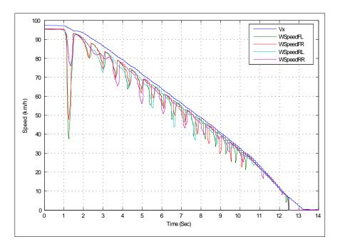
Figure 6.30: Plot of simulated vehicle (Vx) and wheel speeds (WSpeed) on a low friction surface ( $\mu = 0.2$ ) for ABS braking manouevure.
