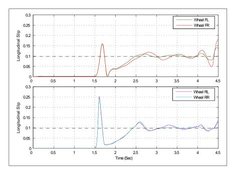
Figure 4.21: Case A : longitudinal slip responses of front and rear wheels with respect to the slip setpoints (dashed line) ; (p = 0.45)
