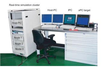
Figure 6.3: Picture of real-time simulation cluster with test bench
