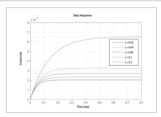
Figure 2.6: Step response of the slip dynamic at constant vehicle speed of 60 km/h for slip value from 0.02 to 0.2
