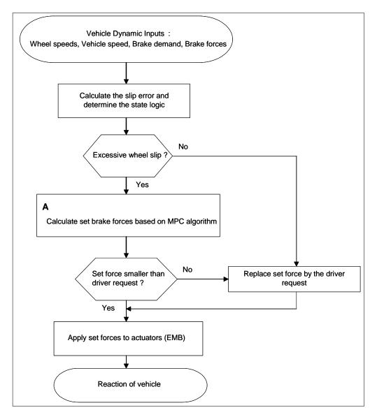
Figure 3.4: Wheel slip control algorithm structure
