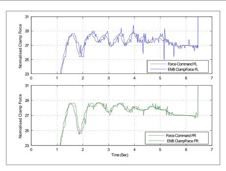
Figure 6.14: Amplified view of measured clamp force responses by the front EMB calipers to the force command input
