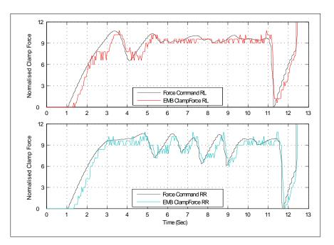
Figure 6.20: Amplified view of rear EMB clamp force response to the force command input
