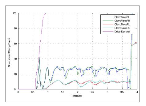
Figure 6.28: Plot of measured clamp forces by EMB brake calipers (ClampForce FL,FR,RL,RR) and driver brake request (Force Demand) during ABS braking for a medium friction surface ( $\mu = 0.5$ )
