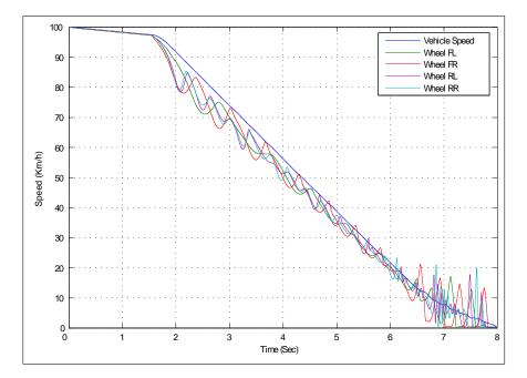
Figure 4.18: Plot of vehicle and wheel speeds on a medium friction surface ( $\mu = 0.5$ ) with p value of 0.8
