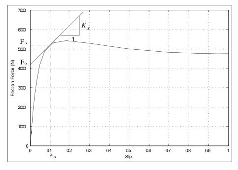
Figure 2.4: Linerisation of slip curve using slip stiffness
