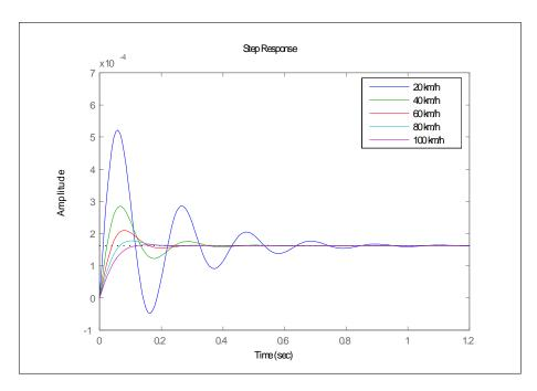
Figure 2.7: Step response of the dynamic slip at slip value of 0.1 for an vehicle speed from 20 to 100 km/h
