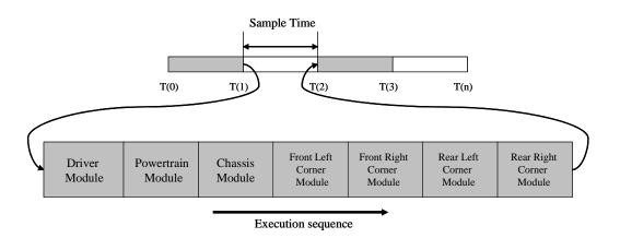
Figure 4.5: An original execution sequence of the vehicle model
