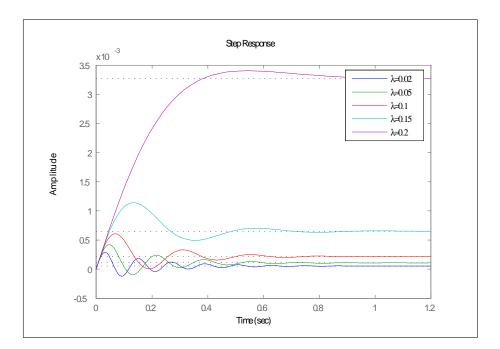
Figure 2.8: Step response of the slip dynamic at constant vehicle speed of 80 km/h for slip value from 0.02 to 0.1
