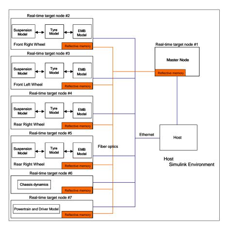
Figure 4.4: Overview of the distributed vehicle simulation model
