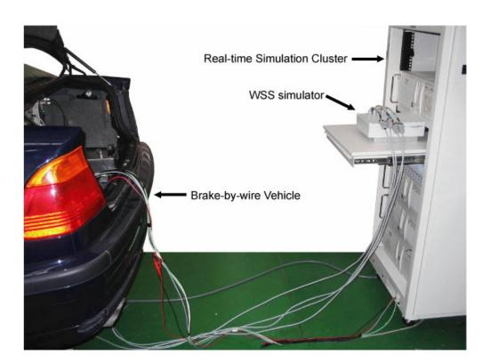
Figure 6.5: Picture of interconnection between the brake-by-wire vehicle, real-time simulation cluster and wheel speed simulator (WSS simulator)
