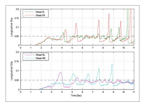
Figure 6.17: Simulated longitudinal slip response of front wheels (FL,RL) and rear wheels (RL,RR) on a high friction surface ( $\mu = 0.2$ ) : Slip set point of 0.05 (dashed line)
