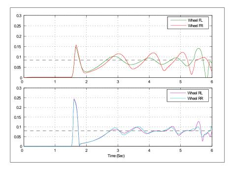
Figure 4.26: Longitudinal slip response of front and rear wheel with respect to the slip setpoint (dashed line) for an ABS braking on a medium friction surface ( $\mu = 0.5$ ); (p = 0.25)
