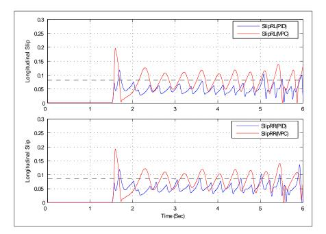
Figure 5.11: Comparison of rear wheel slip response w.r.t optimal slip level (dashed line) of 0.08 on high friction surface ( $\mu = 0.5$ )
