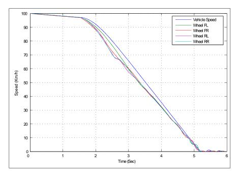
Figure 4.11: Plot of vehicle and wheel speeds on a high friction surface ( $\mu = 0.85$ ) with with p value of 0.2
