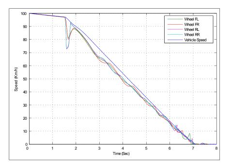
Figure 4.25: Plot of vehicle and wheel speeds during an ABS braking manoeuvre on a medium friction surface ( $\mu = 0.5$ ): a step braking is applied at 1.5 sec; (p = 0.25)
