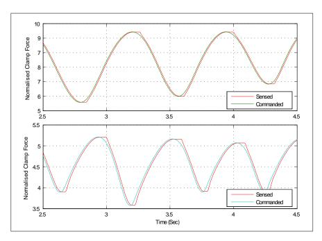
Figure 4.33: Amplified view of responses by the EMB caliper model (sensed) to the commanded clamp force (commanded) from the wheel slip controller : (a) front left brake caliper; (b) rear left brake caliper : Low friction surface ( $\mu = 0.2$ ), (p = 0.25)
