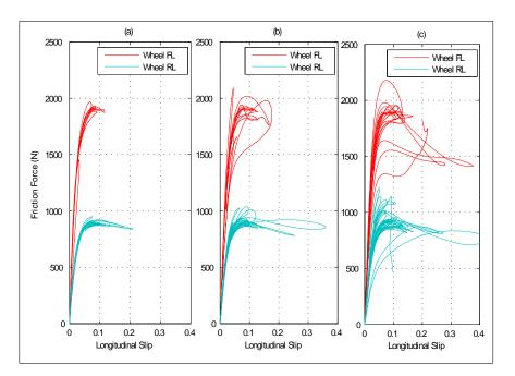
Figure 4.19: Plot of type friction forces vs longitudinal slips on a medium friction surface ( $\mu = 0.5$ ) : (a) p = 0.2 (b) p = 0.4 (c) p = 0.8
