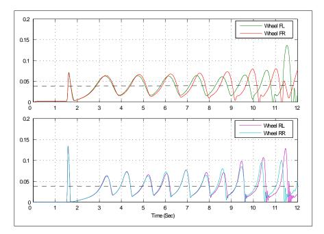
Figure 4.31: Longitudinal slip response of front and rear wheel with respect to the slip setpoint (dashed line) during an ABS braking on a low friction surface ( $\mu = 0.2$ ); (p = 0.25)
