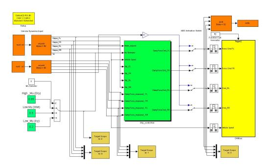
Figure 6.6: Real-time implementation wheel slip control model: reflective memory blockset (orange), CAN communication blockset (yellow) and wheel slip control algorithm block (green)
