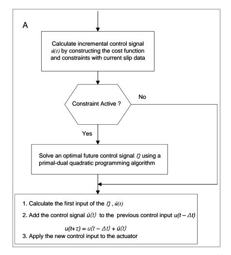
Figure 3.5: Model Predictive Control Strategy : incremental control signal  $\dot{u}(t)$ , future control signal  $\eta$ , control signal u(t).
