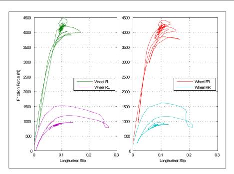
Figure 6.25: Characteristic friction force curve of front and rear wheels for ABS braking stop on high friction surface ( $\mu = 0.85$ )
