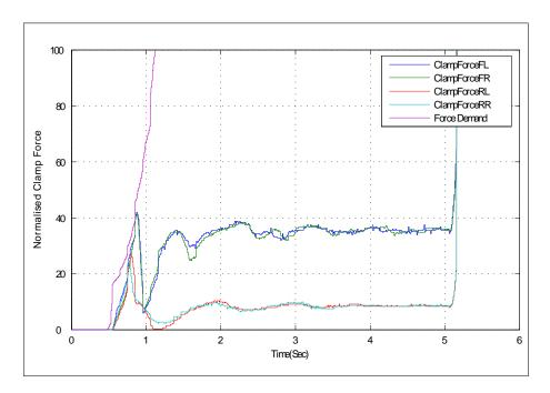
Figure 6.24: Plot of measured clamp forces by EMB brake calipers (ClampForce FL,FR,RL,RR) and driver brake request (Force Demand) during ABS braking for a high friction surface ( $\mu = 0.85$ )
