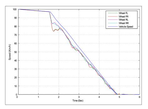
Figure 5.2: Plot of vehicle and wheels speed on a high friction surface ( $\mu = 0.85$ ). Spike braking is applied at 1.5 sec: PID control
