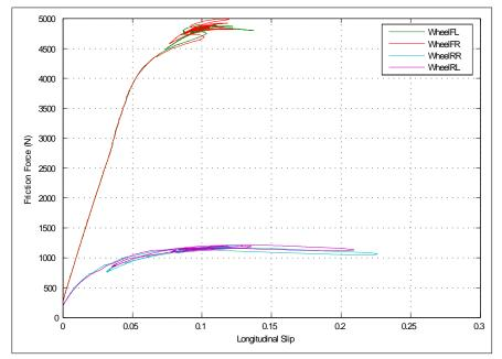
Plot of longitudinal slip vs. tyre friction force on high friction surface ( $\mu = 0.85$ ) under the closed loop MPC control
