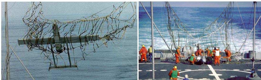
Fig. 2.2 Pioneer UAV net assisted recovery
