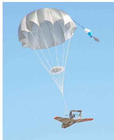
Fig. 2.3 DRS Unmanned Technologies' Neptune UAV with parachute recovery
