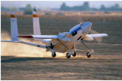
Fig. 2.9 Scorpion free-wing tilt-body UAV
