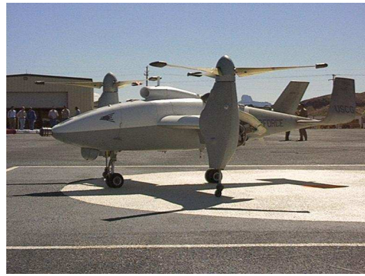
Fig. 2.8 Eagle Eye tilt-rotor VTOL UAV
