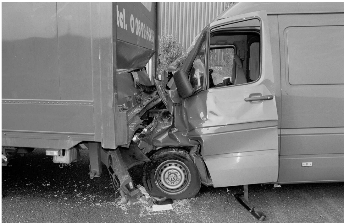
Figure 2 A truck underrun accident - An example of poor geometrical compatibility [62]
