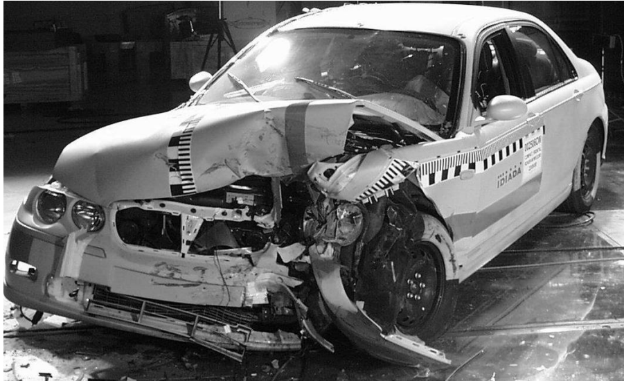
Figure 20 Post crash deformation (Rover 75) – Rover 75 versus small passenger vehicle. Closing velocity 112km/h. Overlap ratio 50% of the width of the smaller vehicle
