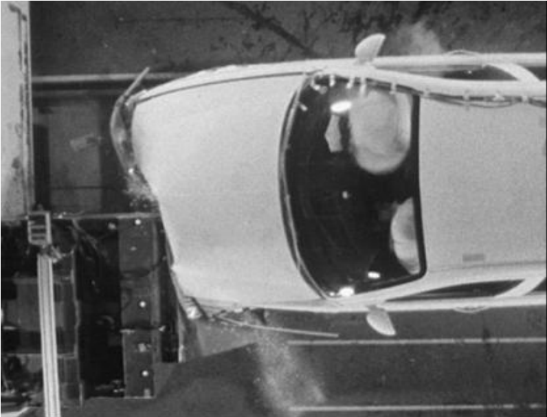
Figure 17 Rover 75 – EURO NCAP Crash Test – 64km/h. Overlap ratio 40%.
