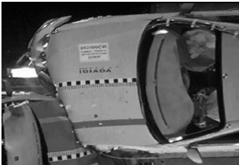
Figure 19 Overhead view - Car-to-car head-on collision – Rover 75 (right) versus small passenger vehicle (left). Closing velocity 112km/h. Overlap ratio 50% of the width of the smaller vehicle
