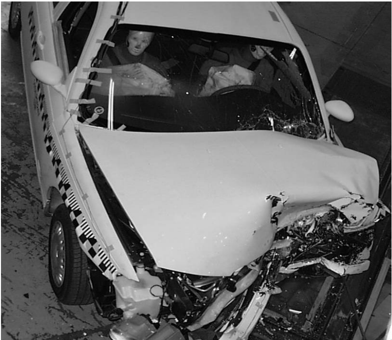
Figure 18 Post-crash deformation (Rover 75) – EURO NCAP Crash Test – 64km/h. Overlap ratio 40%
