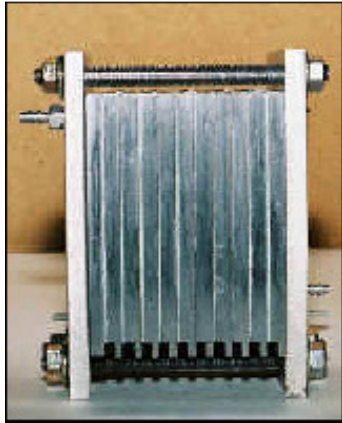
Figure 12 PEMFC 10 cell stack BCS fuel cell at RMIT Renewable Energy Lab.
