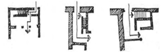
The first indirect entrance type leads the visitors to the guest areas vertically at different levels
