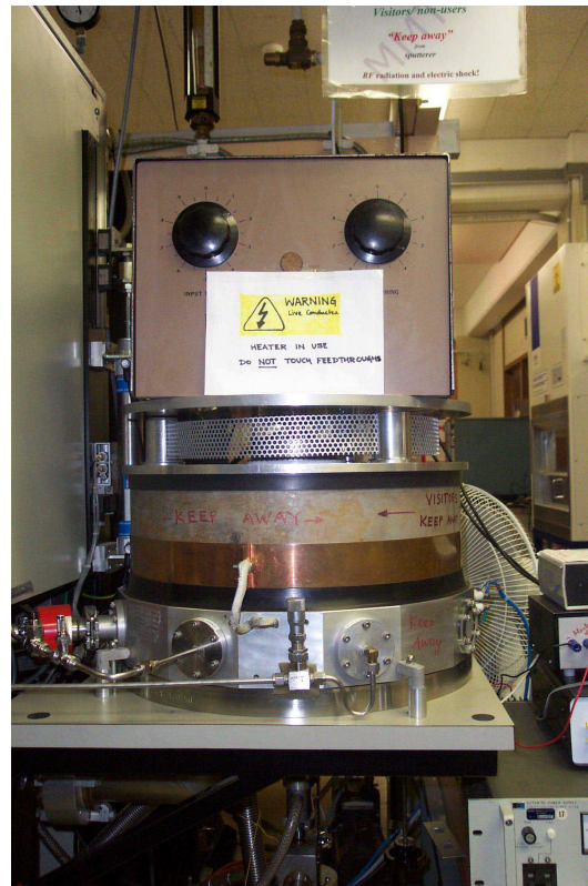
Figure 3.1: View of the vacuum chamber and RF matching box on the RF magnetron sputterer used for BST deposition in the RMIT Vacuum Laboratory.
