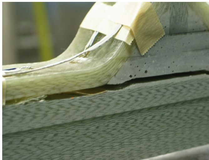
Figure 5-13: Horizontal crack growth along filler region (HDS30)
