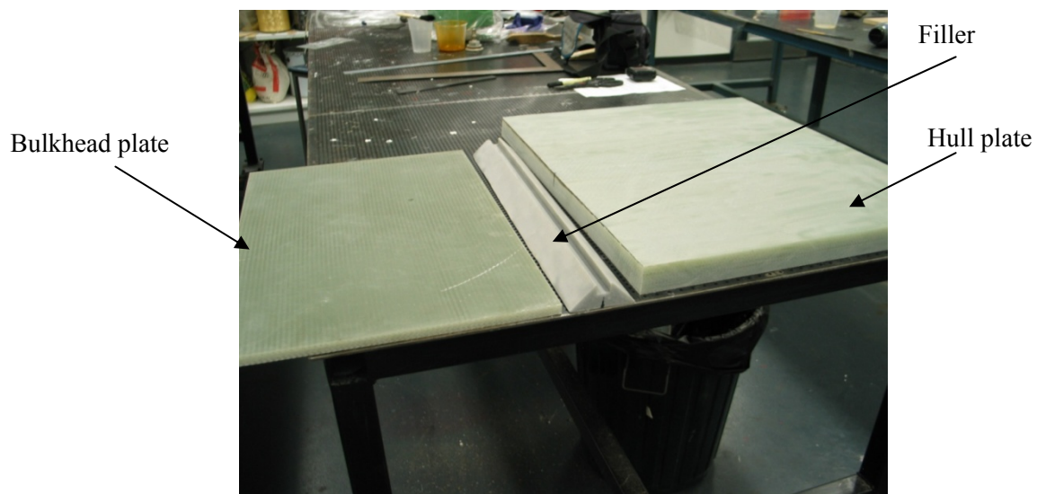
Figure 5-3: Separate T-Joint components
