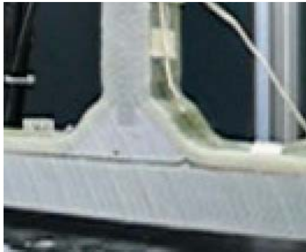
Figure 5-19: Photograph of failed T-joint with a slanted disbond (TJ4.7)
