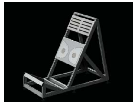
9.11 CAD drawing of new shelf assembly with spreader plates incorporated. Image Steven Curran.
