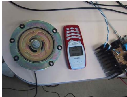
9.08 The vibration actuator removed from a 'rumble pack'. Photographed next to mobile phone.
