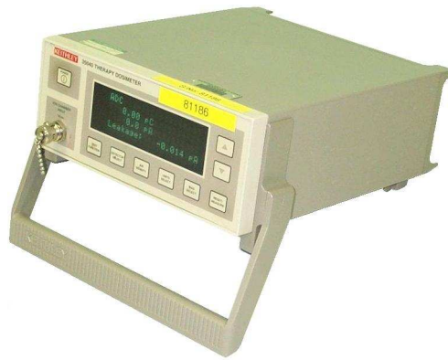
Figure 12. An image of the Keithley model 35040 electrometer. Various menus can be assessed through the front screen shown by the green illuminated panel. Access to the electrometer is obtained either through the front TNC port or at the rear of the device. The base of the device is approximately 50 cm × 50 cm.
