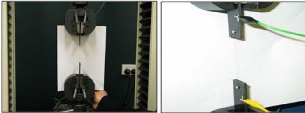
Figure 3.5: Tensile test of SMA wires on UNITED testing machine [17].
