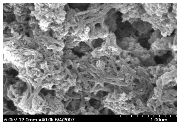
Figure 6.14: SEM image of the polyaniline/diamond nanofibers.
