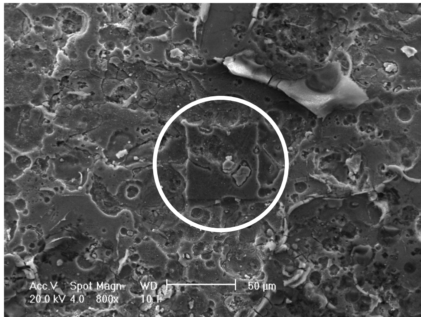
Figure 5-3: SEM micrograph of corroded surface around exposed analysis area, indicated by the circle
