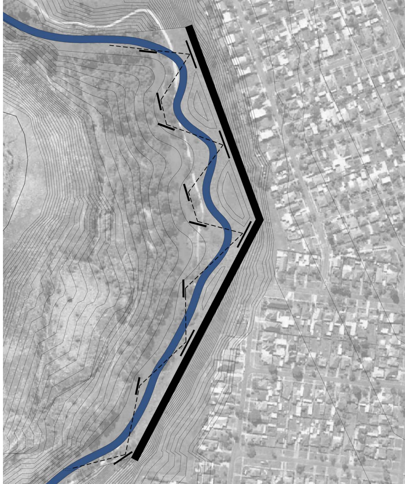
Diagrammatic plan describing the shift in river and increase in force between the existing housing and new river path. This directs the need to provide a barrier which will stop further erosion. The housing in this scenario becomes a thick line that has the potential for up to 8 stories of development.
