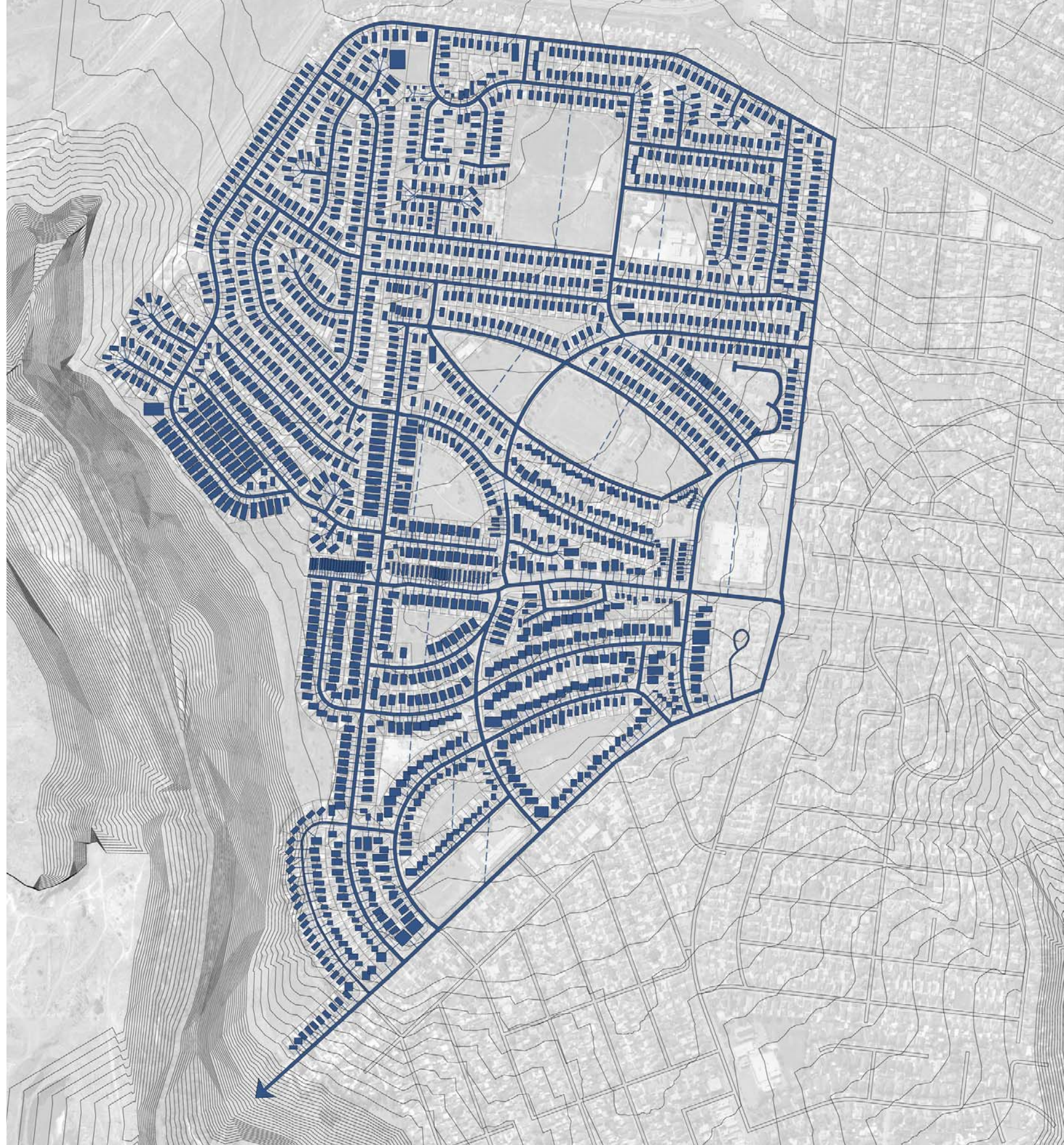
Urban Catchment Plan: Impervious surfaces of rooftops and roads become catchment, distribution and discharge points. The road layout (not the topography) drives the hierarchy of flow.
