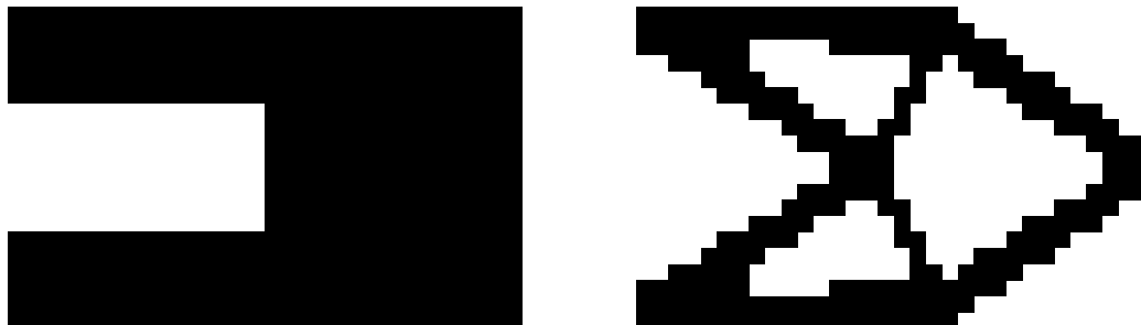
Figure 2.21 The initial guess design and the final topology obtained by the BESO method for the SCB problem.
