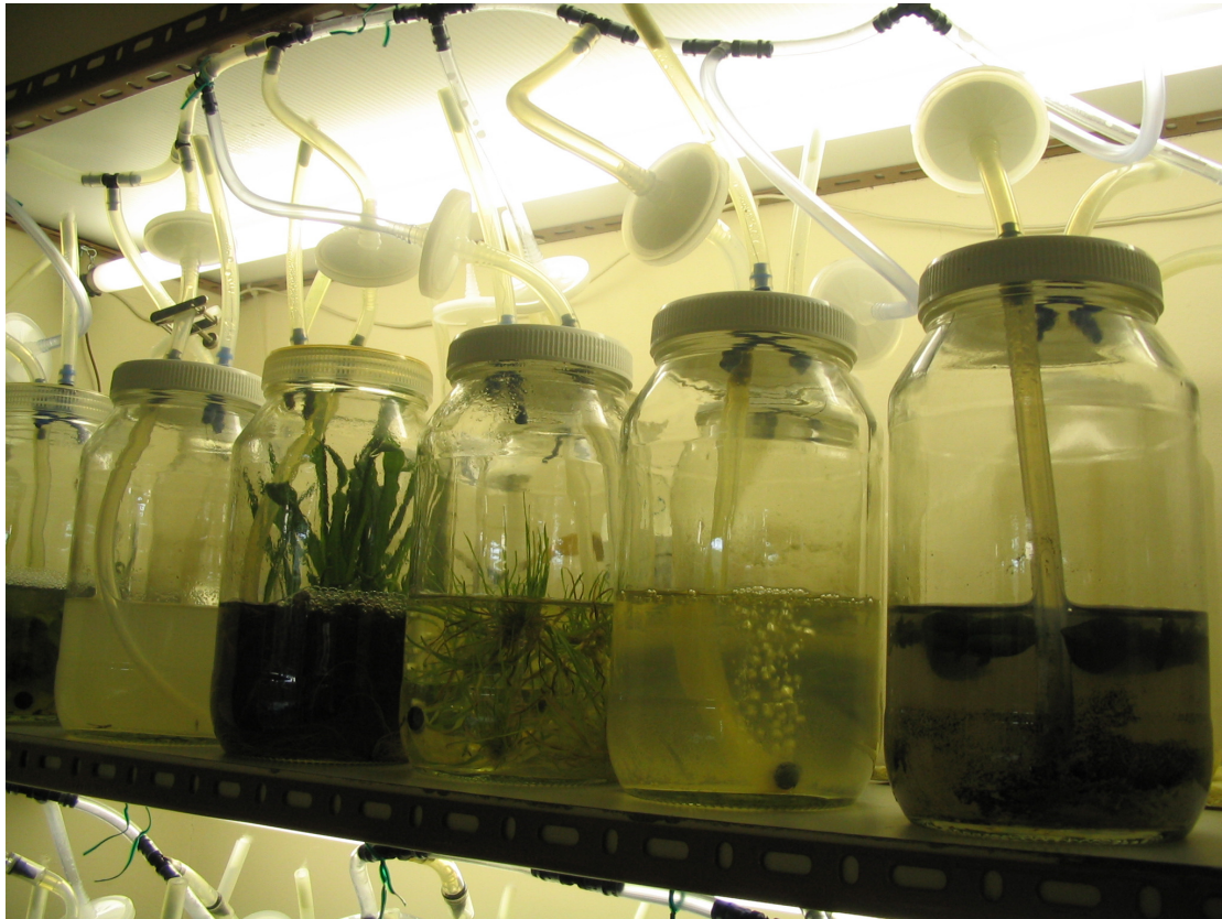
Figure 5-1: Liquid tissue culture of aerated glass jars, joined by sterilised tubing which provides sterile air through micropore filters.
