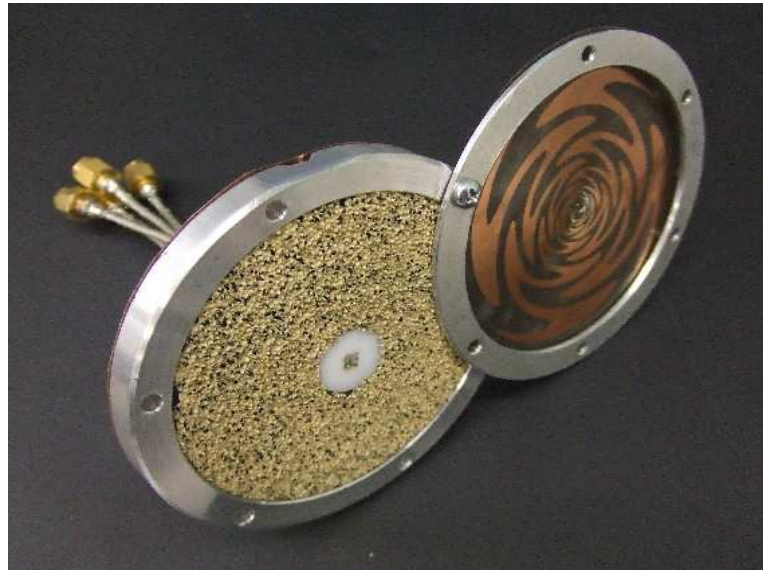
Figure 5.8: Unassembled Sinuous Antenna
