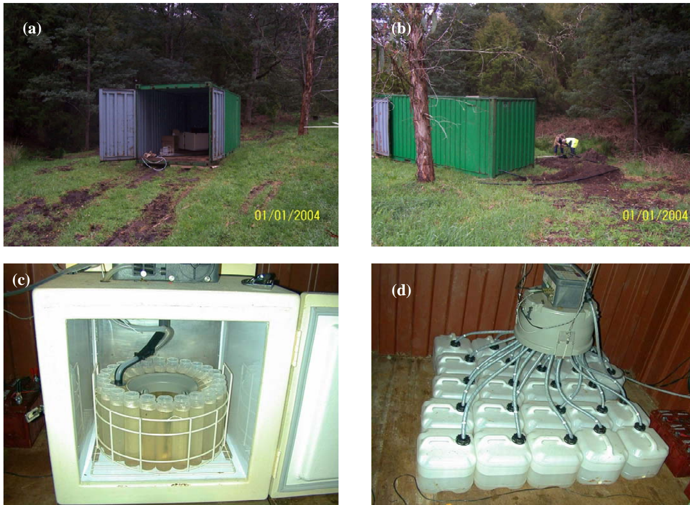
Figure 3.3 - The event sampler on the East branch
