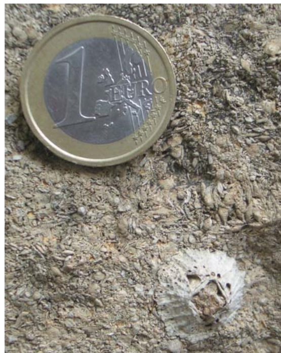
Figure 4 Tetraclitella sp., to the lower right of the one-euro coin, sitting proud in its Batesford Limestone matrix. Photograph taken on 29 January 2006, several months before removal from a column in Building 20, RMIT University (Old Magistrates’ Courts), Russell Street frontage, Melbourne. The diameter of the coin is 23.25 mm.
