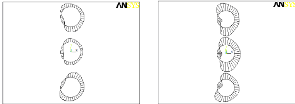
(a) Symmetrical gap flows at t=11.2 s (b) asymmetrical gap flows at t=13.9 s Figure 10. Instantaneous pressure distribution around the three cylinders
