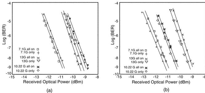
Fig. 4. Measured BER performance for three SCM channels, using remote LO delivery and optical filtering via (a) two cascaded FBGs or (b) a single eight-phase-shifted FBG.
