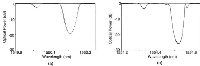
Fig. 2. Measured transmission responses of FBG designs for LO recovery. (a) Two concatenated FBGs and (b) single novel FBG structure with eight phase shifts of  $64^\circ$ .
