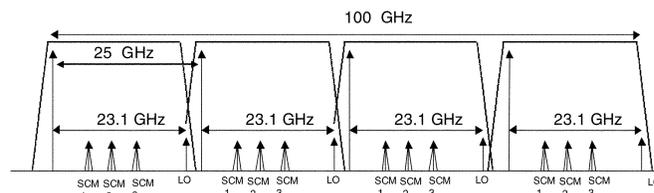
Fig. 1. Wavelength allocation scheme for a spectrally efficient WDM fiber-radio network incorporating simultaneous SCM and remote LO delivery.
