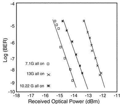
Fig. 5. Measured BER performance for three SCM channels, using remote LO delivery and optical filtering via a 25-GHz dispersion-flattened FBG in conjunction with an eight-phase-shifted FBG.
