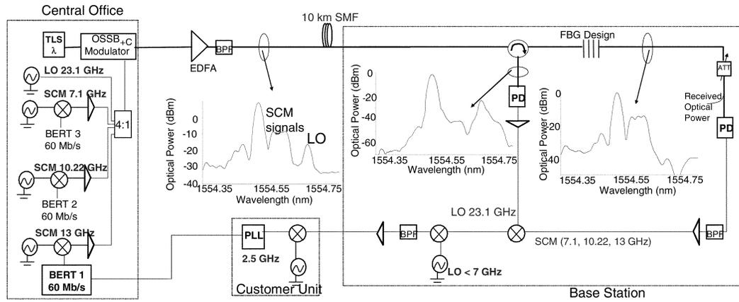
Fig. 3. Experimental setup to demonstrate simultaneous delivery and recovery of a remote LO and three IF SCM data signals, in a 25-GHz band, using novel FBG optical filtering techniques.
