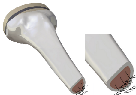
Figure 4.8: Constraint and applied loads on the models
