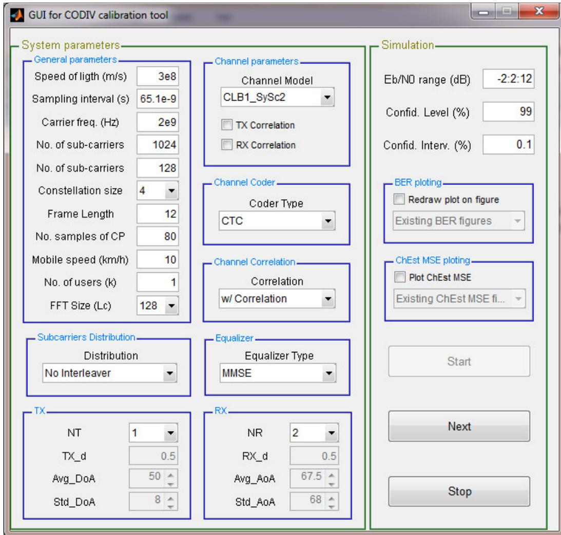
Figure 23 - Simulation window
