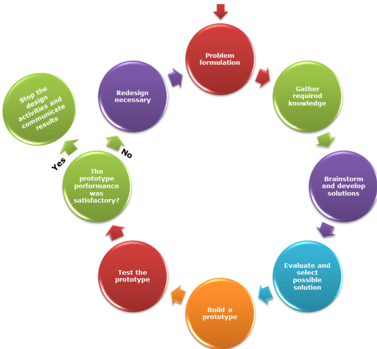
Figure 3.1. Iterative steps in the design process of a milliliter scale bioreactor with the problem formulation step as the starting point.
