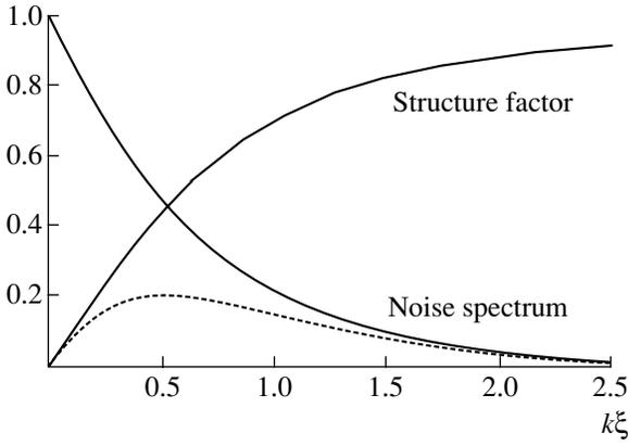
**Fig. 4.** Static structure factor  $S(k; n_c)$  (homogeneous condensate with density  $n_c$ ), noise spectral density  $S_V(k)$ , and effective excitation rate  $S(k; n_c)S_V(k)$  (dashed solid line) vs. quasiparticle wave vector  $k$ . The noise spectrum is the Fourier transform of the correlation function (5) with a correlation length  $l_{\text{corr}} = 1.5\xi$ ; it is normalized to  $S_V(k=0) = 1$ . Wave vectors are normalized to the inverse healing length  $1/\xi = \sqrt{4gn_c}$ .
