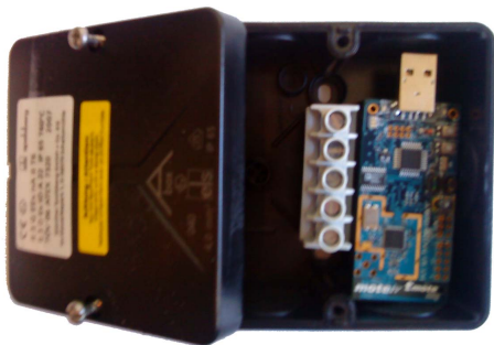
Fig. 5. ATEX case with a sensor node.
