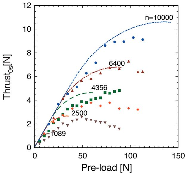
Fig. 7 Output force characteristics of 20  $\mu\text{m}$  diameter sliders by changing the numbers of projections from 100 by 100 to 33 by 33;  $n=10000$  ( $\bullet$ ), 6400 ( $\blacktriangle$ ), 4356 ( $\blacksquare$ ), 2500 ( $\blacklozenge$ ), and 1089 ( $\blacktriangledown$ ).
