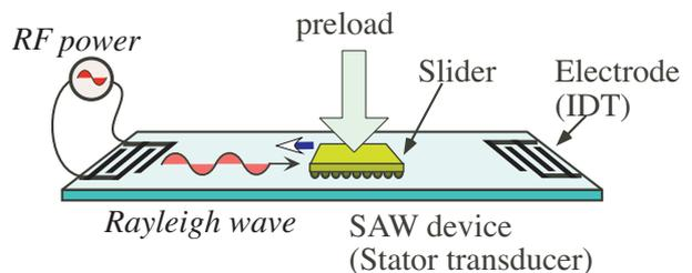
Fig. 1 Schematic of surface acoustic wave motor.
