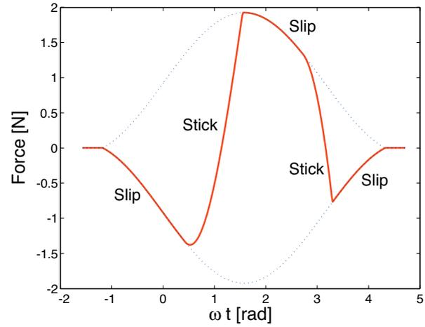
Fig. 6 Force transmission from stator surface to slider with stick and slip.
