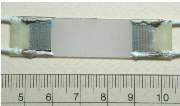
Fig. 4 Photo of SAW transducer for linear motor at 9.6 MHz driven by single electrical source.
