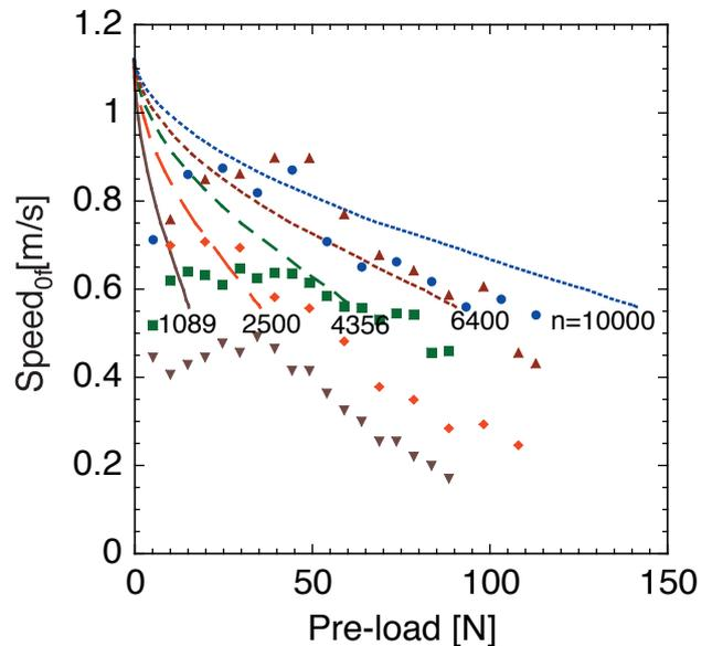
Fig. 8 No-load speed characteristics of 20  $\mu\text{m}$  diameter sliders by changing the numbers of projections from 100 by 100 to 33 by 33;  $n=10000$  ( $\bullet$ ), 6400 ( $\blacktriangle$ ), 4356 ( $\blacksquare$ ), 2500 ( $\blacklozenge$ ), and 1089 ( $\blacktriangledown$ ).
