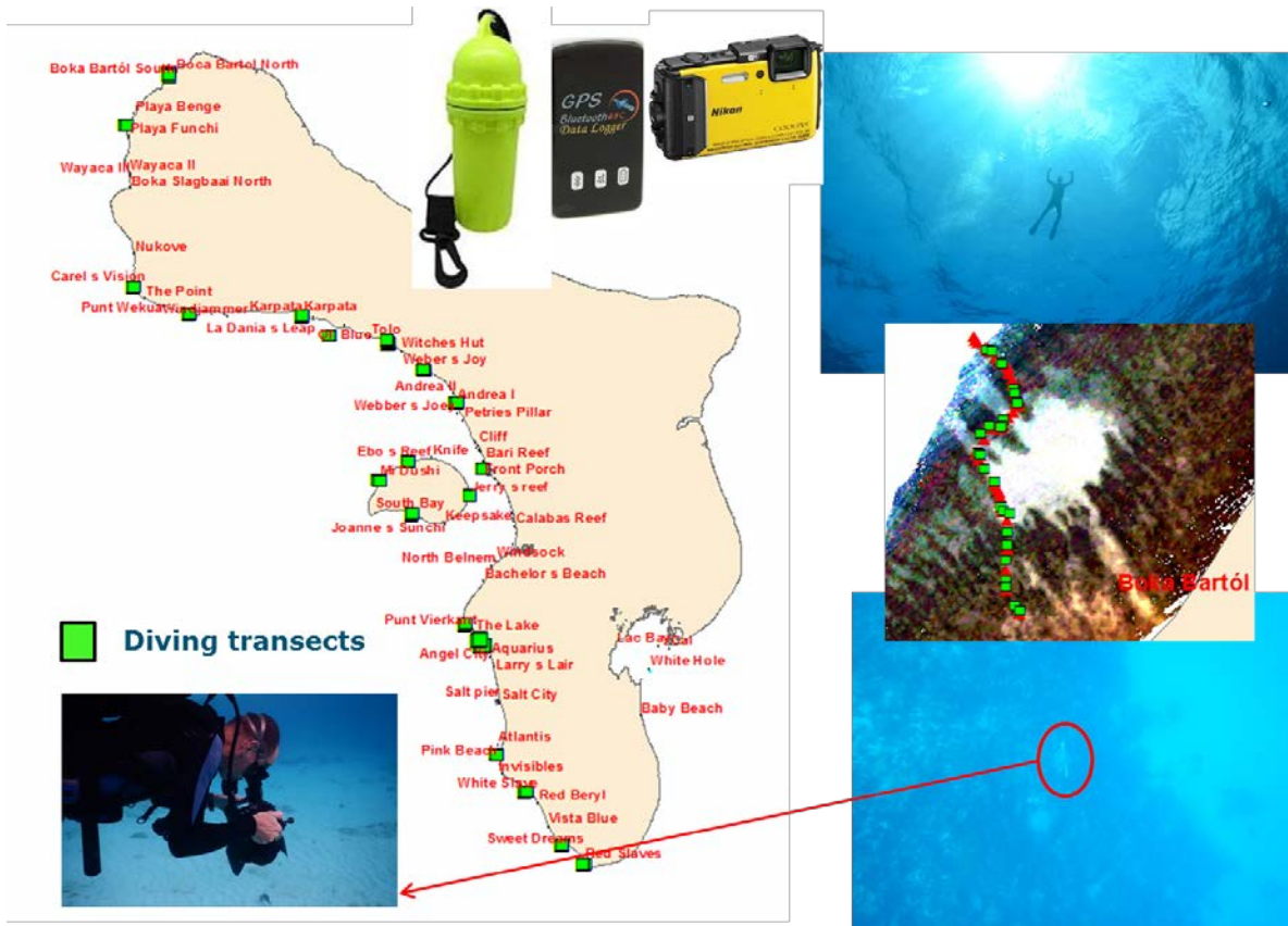
Figure 26. 20 GPS diving transects were collected in June 2016. Geotagged pictures were created by one person snorkelling at the water surface with a GPS in a plastic floating box following exactly above the divers taking pictures at the sea bottom.
