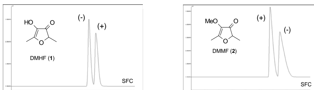
Figure 2. Optical Resolution by Enantioselective CO 2 SFC.
