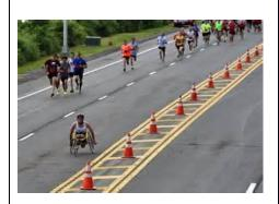
Racing wheelchairs are used for taking part in road races and marathons. These three wheel chairs are designed to travel on smooth surfaces. There are no gears and the athlete's arms are continuously pushing the chair on the smaller designed push rims.
