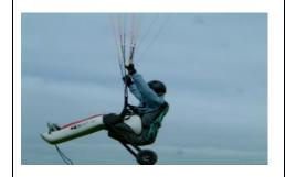
A device called the Phoenix is a custom-made wheelchair in the place of a normal harness.
