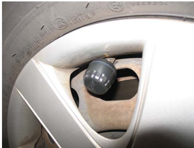
Figure 4-6: Tyre pressure gauge with the RF transmitter installed on Mazda 3 tyre
