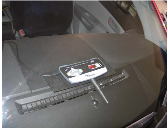
Figure 4-7: Instrument Panel to receive, indicate and record tyre pressure values
