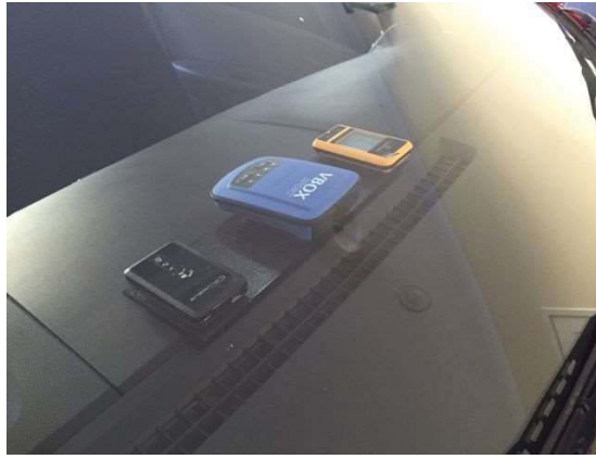
Figure 5-9: Installation of GPS receivers on a dashboard
