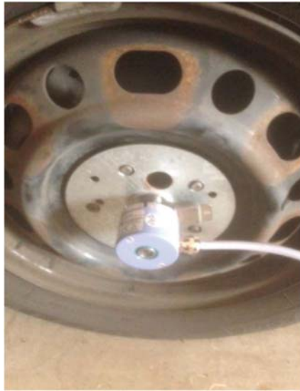
Figure 3-7: Installation of the Encoder WGD 58H on Mazda 3
