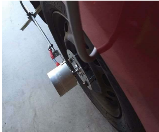
Figure 3-25: Full installation of the Encoder on Mazda 3 with sunlight / rain protection
