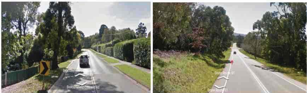
Figure 7-8: Examples of the environments where the Novatel ProPak-V3-L1 with 10° mask angle generated the outliers during the kinematic Test No4
