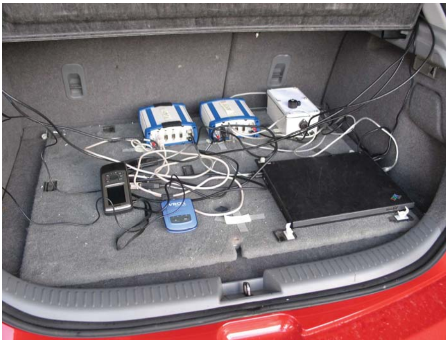
Figure 5-10: GPS receivers and speed measurement system in the boot
