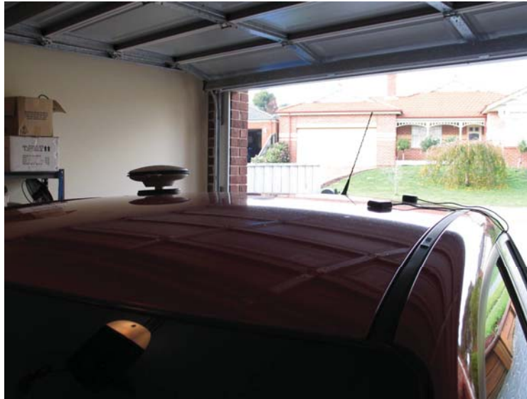
Figure 5-11: GPS antennas on the roof
