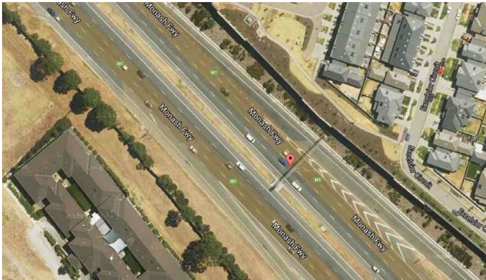
Figure F.1: An outlier of Novatel with a 10° elevation mask around a road gantry (Speed error = 12.6 km/h, Number of satellites in view = 5, HDOP = 3.5)
