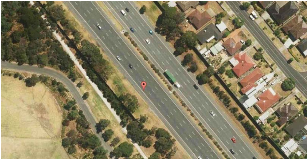
Figure 6-11: An outlier generated by G-Log (Speed error = 2.0 km/h, Number of satellites in view = 11, HDOP = 0.85)
