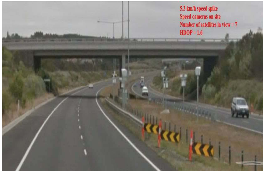
Figure 5-16: Example of the environment where an outlier was generated by Novatel ProPak-V3-L1
