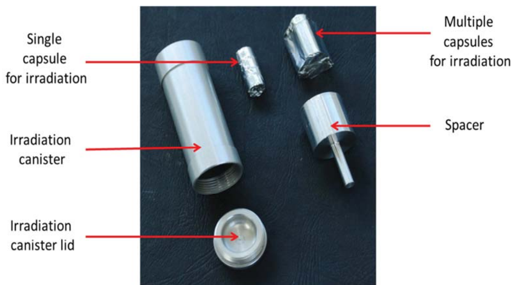
Figure 6-6. The irradiation setup used for neutron bombardment of the AuNPs.
