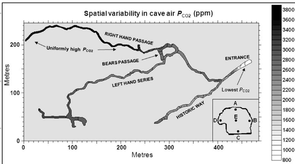
To produce the most accurate map of spatial cave air  $P_{CO_2}$  and temperature values possible, measurements were taken at several points along the passage cross-section at every location (Fig.2, inset). These values were then averaged to produce the x-y cave-scale survey.
