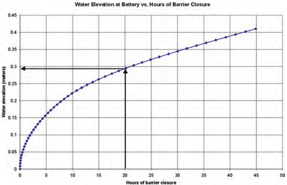
Figure 4.4. Rising water levels behind the closed barrier system at the Battery in relation to the hours of barrier closure (adapted from Bowman et al. , 2005).
