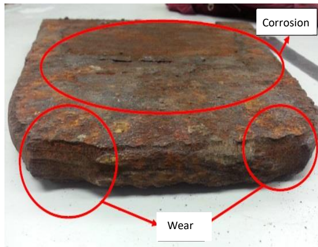
Figure 1.1: Wear and corrosion area of the blade after three months' operation
