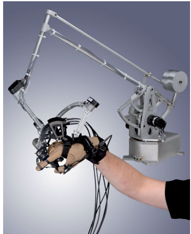
FIGURE 12 | CyberForce: haptic device with exoskeleton. A virtual environment can be interacted with haptically. Image courtesy of CyberGlove Systems LLC.
