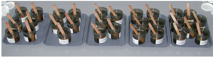
FIGURE 4 | Cups with silicone oils ranging from very thin to highly viscous, used for viscosity discrimination experiments.
