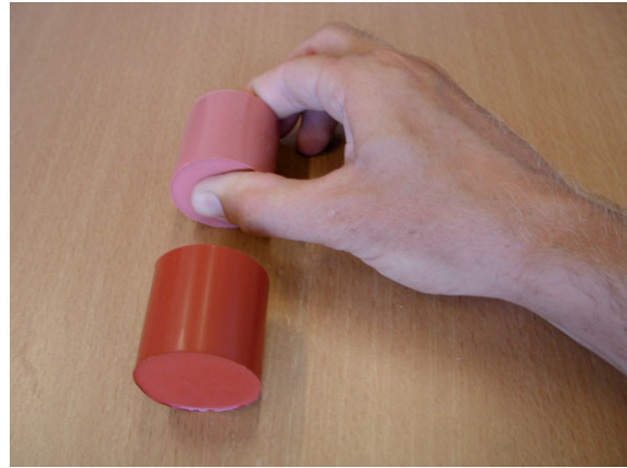
FIGURE 2 | A blindfolded subject compares the compliance of two silicon rubber cylinders in a discrimination experiment.
