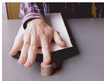
FIGURE 11 | Experimental set-ups for curvature after-effect measurements. Left: A blindfolded observer touches an adaptation surface with his index finger. Right: The same observer dynamically explores the curvature of a surface. Both conditions give rise to curvature after-effects. The dynamic case even transfers to the other hand.
