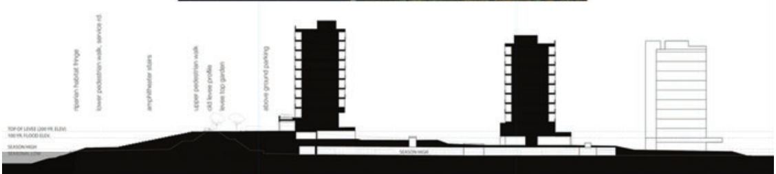
Figure 7.1. Super-levée on the Edogawa in Tokyo (top). Source: William Verbeek. Cross-section through a super-levée in Osaka (bottom). Source: Stalenberg (2010).
