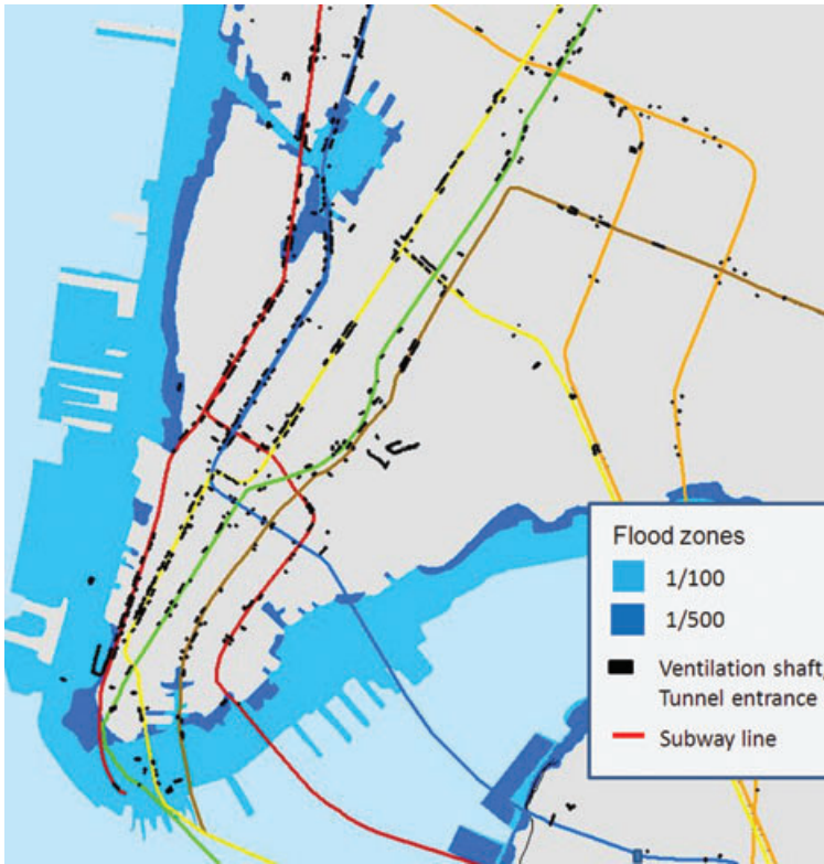
Figure 3.9. Subway lines (colors) and railroad tracks (black) in Manhattan and Brooklyn overlaid with the 1/100 and 1/500 flood zones. Ventilation shafts, subway, and tunnel entrances are depicted in small black rectangles. Source: NYC-DoITT, see Appendix C.
