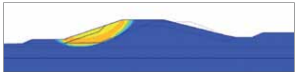
Figure 6.5. Example of sliding at the GEO-08/228-S7 test bore (consolidated LW Plaxis)
