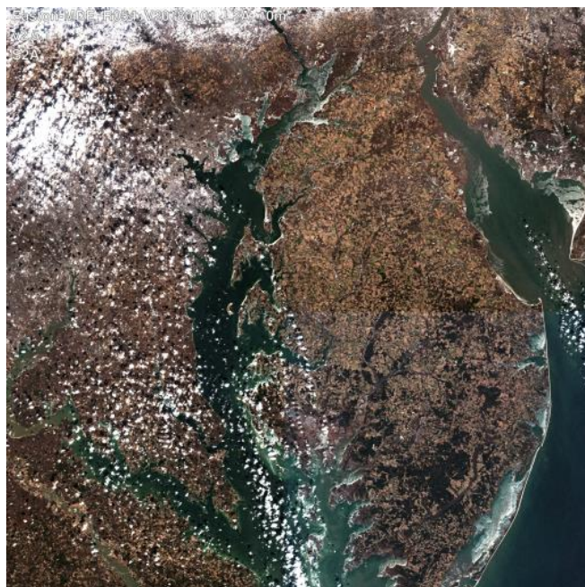
Figure 3: Sentinel-2A L2A image composed of four tiles (from upper left to lower right: T18SUJ, T18SVJ, T18SUH, T18SVH). Lower right tile T18SVH appears brighter than the three others tile due to different AOT content estimates.
