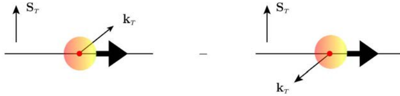
Figure 1.4: The Sivers effect describes a transverse momentum distribution that is anti-symmetric with respect to the proton's spin direction.
