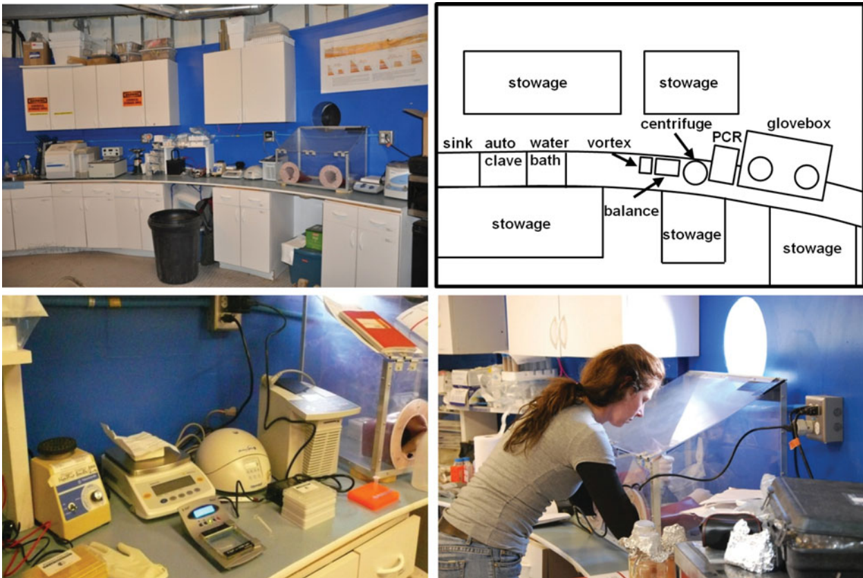
Fig. 1. A view of the biology laboratory on the lower deck floor. The upper panel shows the organization of the molecular biology section deployed in the habitat laboratory. The upper right picture shows a scheme of the arrangement of instruments. The lower panel shows a more detailed view of the instruments. (Photo: EuroGeoMars crews 76–77.)
